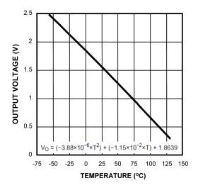
Figure 5. Output Voltage vs Temperature
