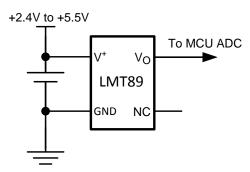
Figure 4. Full-Range Celsius (Centigrade) Temperature Sensor (−55°C to 130°C) Operating from a Single Li-lon Battery Cell
