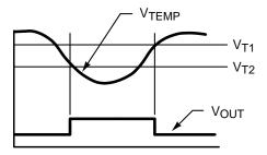
Figure 7. Thermostat Output Waveform
