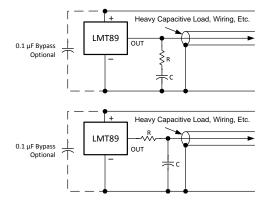
Figure 3. LMT89 With Filter for Noisy Environment and Capacitive Loading Greater Than 300 pF
