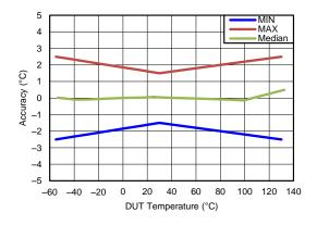
Figure 1. Temperature Sensor Accuracy
