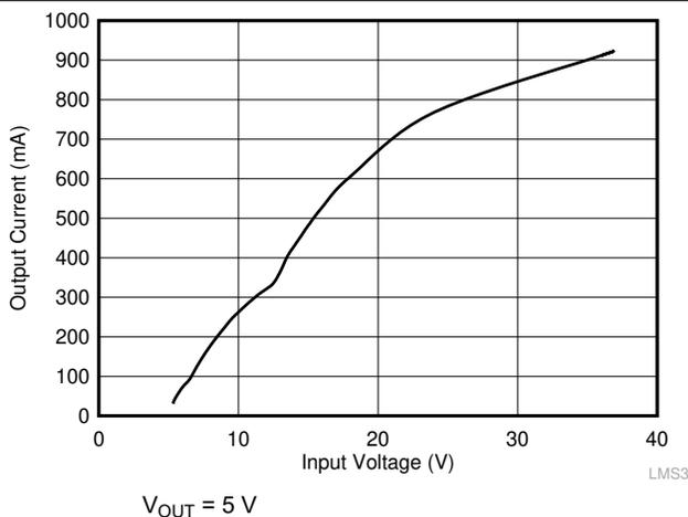
图 9-9. Load Current for PFM-to-PWM Transition
