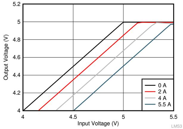
图 8-10. Overall Dropout Characteristics ( $V_{OUT} = 5$  V)
