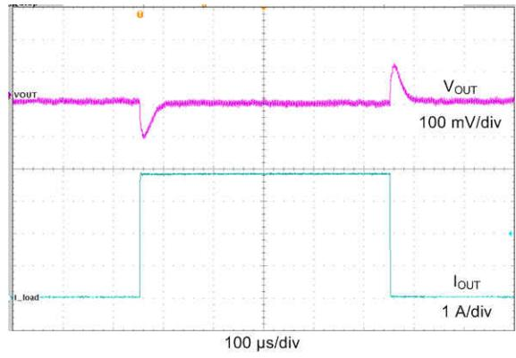
FPWM                       $V_{OUT} = 6\text{ V (ADJ)}$                        $L = 10\ \mu\text{H}$ ,
