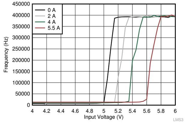
图 8-11. Frequency Dropout Characteristics ( $V_{OUT} = 5$  V)
