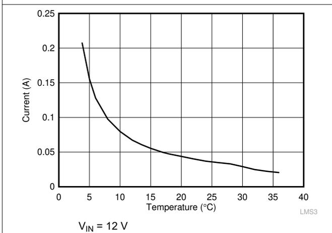
图 7-5. Short Circuit Average Input Current for LMS3635-Q1
