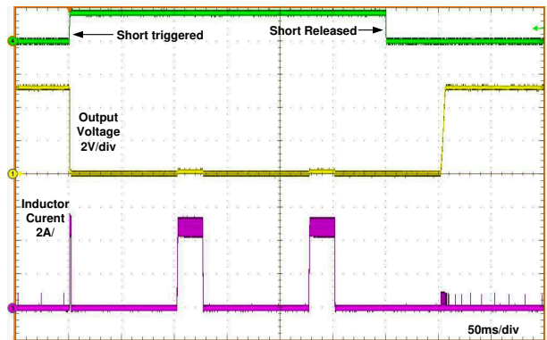
图 8-6. Short-Circuit Transient and Recovery
