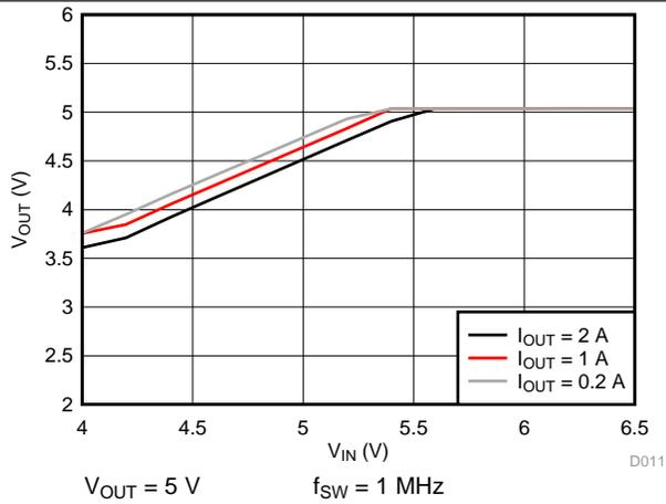
Figure 7. Dropout Curve
