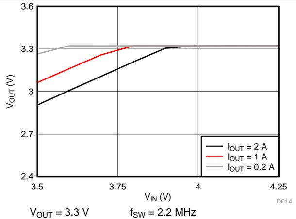
Figure 10. Dropout Curve
