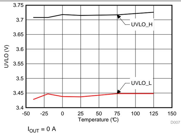
Figure 12. UVLO Threshold
