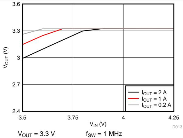
Figure 9. Dropout Curve
