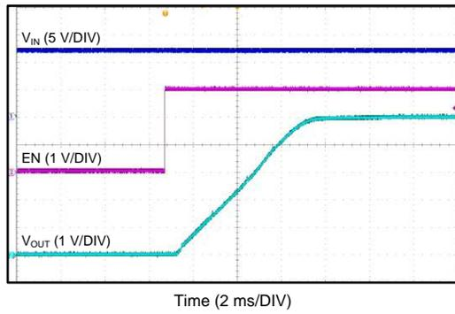
$V_{IN} = 12\text{ V}$        $V_{OUT} = 5\text{ V}$        $I_{OUT} = 1\text{ A}$
