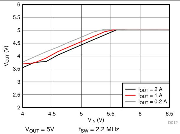
Figure 8. Dropout Curve
