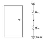
图 8-6. Setting Output Voltage for Adjustable Output Variant
