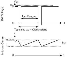
图 8-10. Current Limit Waveforms
