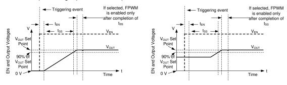
图 8-7. Soft Start with and Without Pre-bias Voltage
