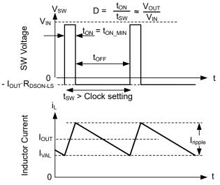
In valley control mode, minimum inductor current is regulated, not peak inductor current.
