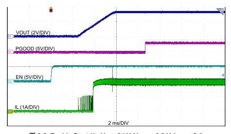
图 8-3. Enable Start-Up  $V_{IN}$  = 24 V,  $V_{OUT}$  = 3.3 V,  $I_{OUT}$  = 2 A
