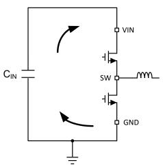
图 9-12. Current Loops with Fast Edges
