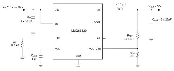
图 9-1. Application Circuit - 5 V (Fixed), 3 A, 400 kHz
