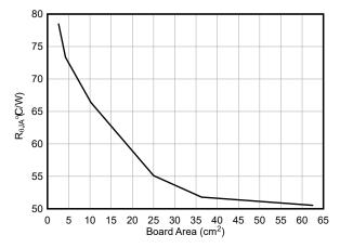
The device operating conditions are as follows: 12-V<sub>IN</sub>, 3.3-V<sub>OUT</sub>, 3-A load, 2.2-MHz, 23°C ambient. 4 layer board, GND plane on Mid-Layer One, 2.8-mil thick copper on each layer, see *LMQ66430-Q1 Buck Controller Evaluation Module User's Guide* for copper pattern and thermal vias.
