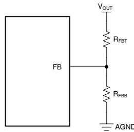
**图 8-6. Setting Output Voltage for Adjustable Output Variant**
