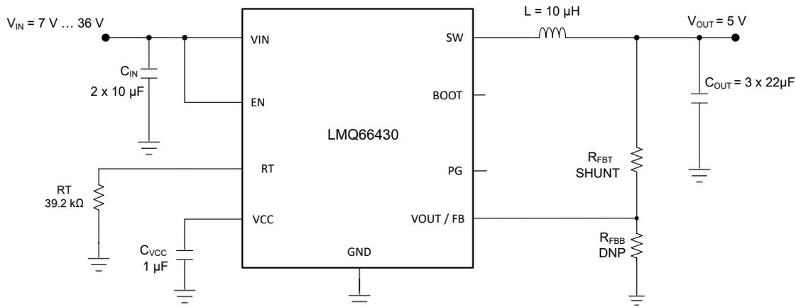
**图 9-1. Application Circuit - 5 V (Fixed), 3 A, 400 kHz**
