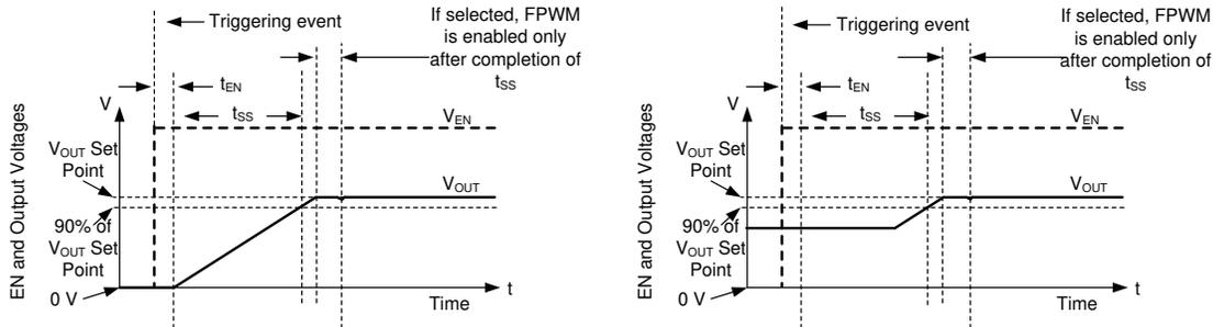
图 8-7. Soft Start with and Without Pre-bias Voltage
