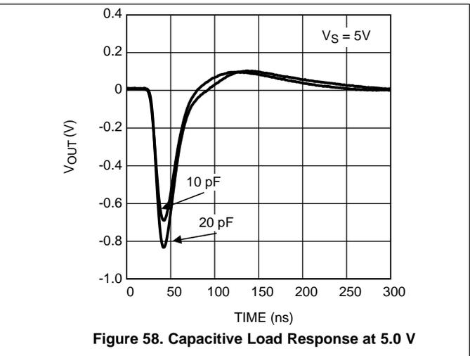
Figure 58. Capacitive Load Response at 5.0 V
