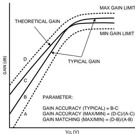
Figure 43. LMH6504 Gain Accuracy & Gain Matching Defined
