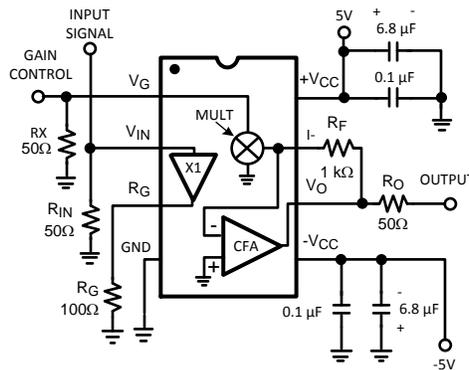
Figure 42. LMH6504 Typical Application and Block Diagram
