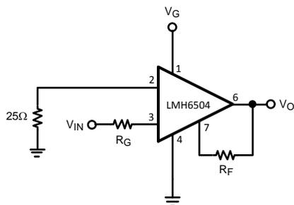
**Figure 45. Inverting Amplifier**
