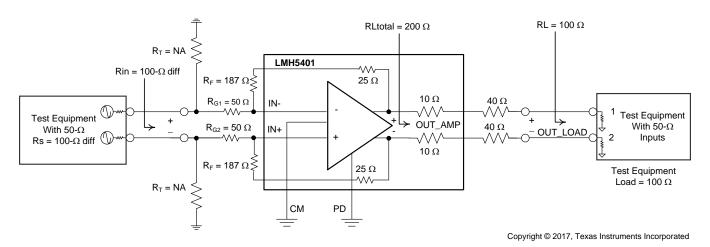
图 55. Test Schematic: Differential Input, Differential Output, G<sub>V</sub> = 4.25 V/V
