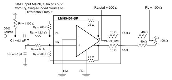
图 59. AC-Coupled, Single-Ended Source to a Differential Gain of a 7-V/V
