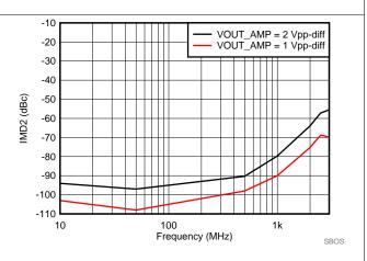
图 22. SE-DE 2nd Order Intermodulation Distortion vs Frequency
