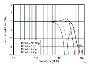
图 66. Frequency Response with Capacitive Load
