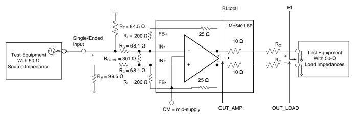
图 61. Noise Gain Compensation for Stability at Gp = 0 dB
