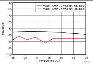
图 20. SE-DE 2nd Order Harmonic Distortion vs Temperature
