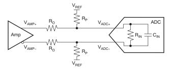
图 69. Resistor Network to DC Level-Shift Common-Mode Voltage
