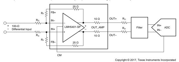
图 67. Differential ADC Driver Block Diagram
