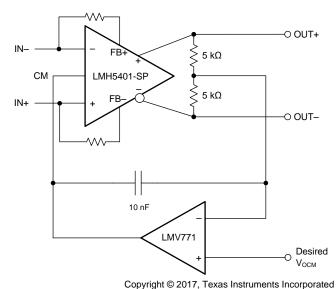
图 71. Common-Mode Correction Circuit
