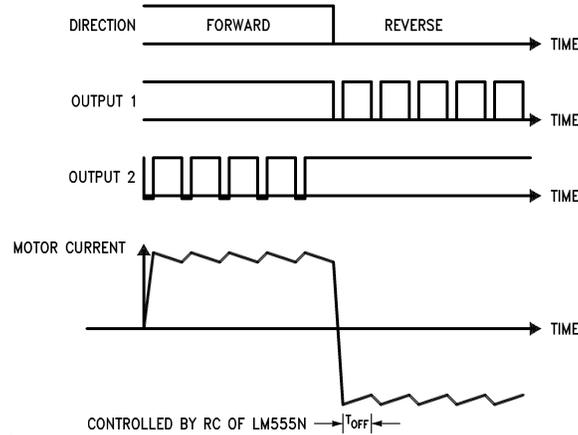
Figure 11-7. Switching Waveforms
