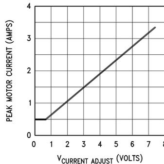
Figure 11-9. Peak Motor Current vs Adjustment Voltage
