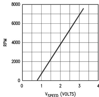
Figure 11-11. Motor Speed vs Control Voltage
