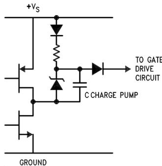
**Figure 11-4. Internal Charge Pump Circuitry**
