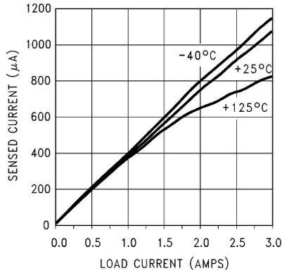
Figure 9-7. Current Sense Output vs Load Current
