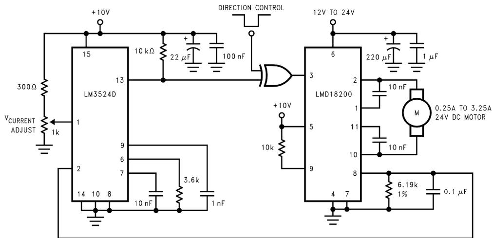
Figure 11-8. Locked Anti-Phase Control Regulates Torque
