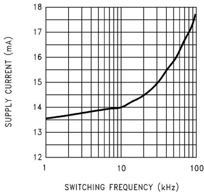
**Figure 9-5. Supply Current vs Frequency ( $V_S = 42V$ )**
