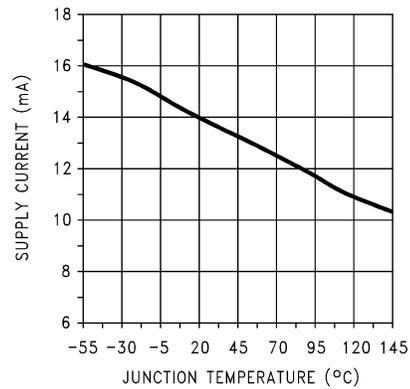
**Figure 9-6. Supply Current vs Temperature ( $V_S = 42V$ )**
