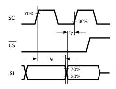
Figure 6. Data Input Timing Diagram
