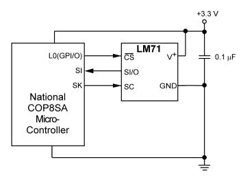
Figure 3. COP Microcontroller Interface
