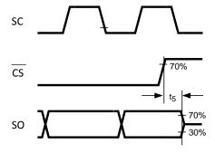
Figure 5. TRI-STATE Data Output Timing Diagram
