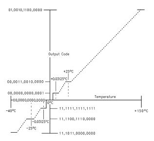
Figure 7. Temperature-to-Digital Transfer Function (Non-linear scale for clarity)
