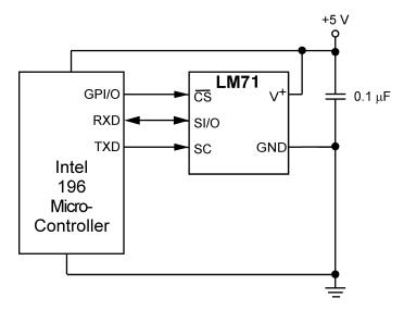
Figure 14. Temperature monitor using Intel 196 processor
