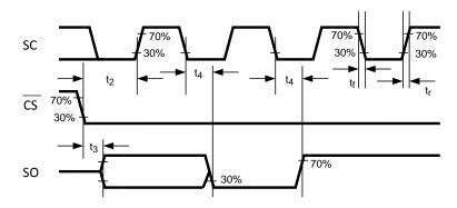
Figure 4. Data Output Timing Diagram
