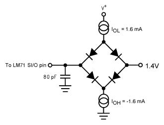
Figure 8. TRI-STATE Test Circuit
