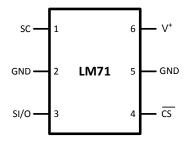
Figure 1. 5-Pin SOT-23 See Package Number DBV
