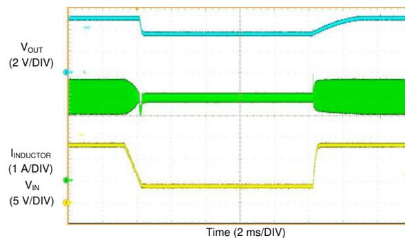
图 9-10. Recovery From Dropout ( $V_{OUT} = 5\text{ V}$ ,  $I_{OUT} = 4\text{ A}$ ,  $V_{IN} = 13.5\text{ V}$  to  $4\text{ V}$  to  $13.5\text{ V}$ )
