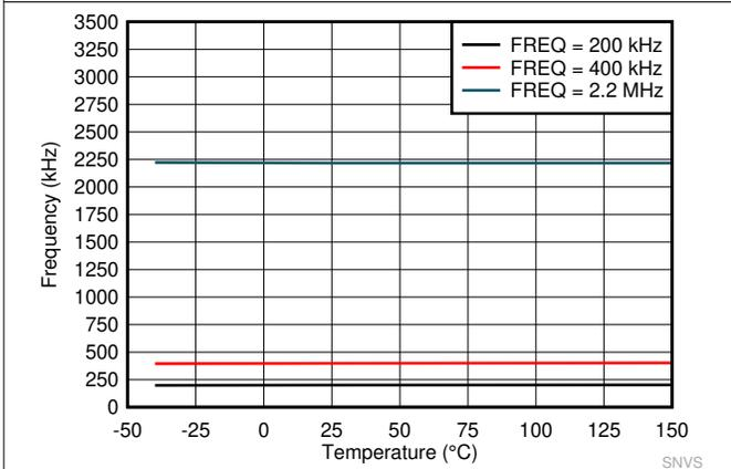
图 8-5. Switching Frequency Set by RT Resistor
