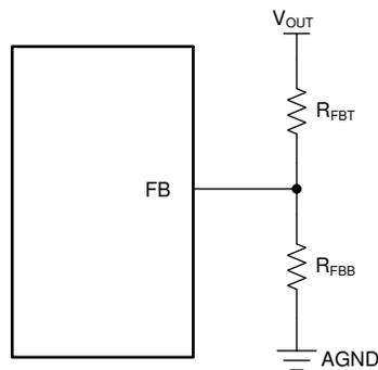
图 9-11. Setting Output Voltage of Adjustable Versions
