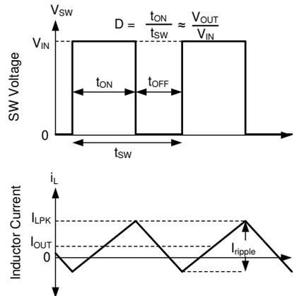
In FPWM mode, Continuous Conduction (CCM) is possible even if  $I_{OUT}$  is less than half of  $I_{ripple}$ .
