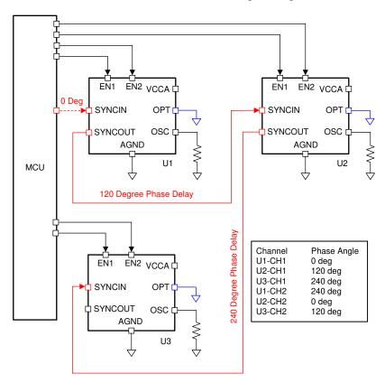
图 8-23. Six Phases 120° Interleaving Configuration
