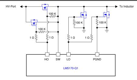
图 9-10. Paralleled MOSFET Configuration
