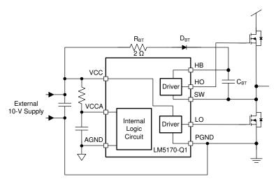
图 8-8. Bootstrap Circuit for High-Side Bias Supply
