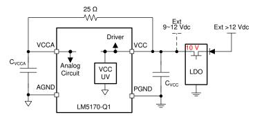
图 8-1. VCC Bias Supply Connections
