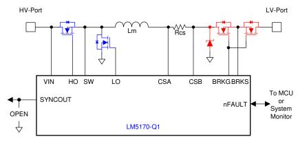
图 8-15. Controlling Dual-Channel Circuit Breaker for MOSFET Failure Protection
