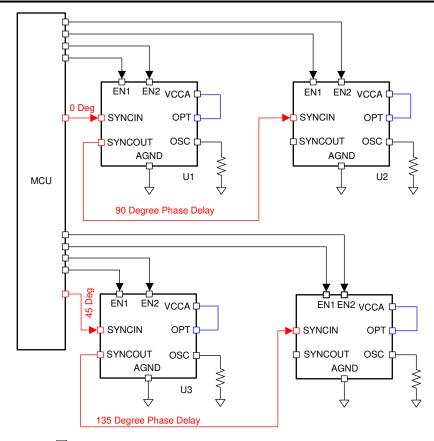
图 8-24. Eight Phases 45° Interleaving Configuration
