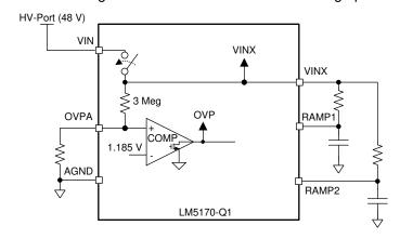
图 8-2. VIN and VINX Pins Configuration
