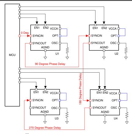
图 8-25. Eight Phases 90° Interleaving Configuration
