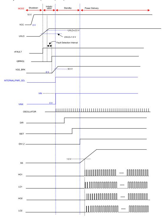
图 9-1. Typical Turnon Sequence Key Waveforms
