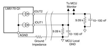
图 8-6. Channel Current Monitor
