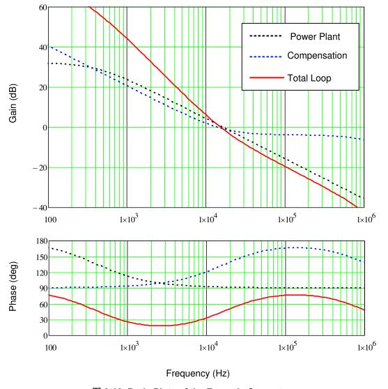
图 9-12. Bode Plots of the Example Converter
