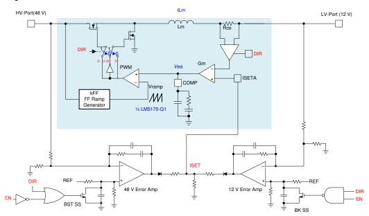
图 9-6. Analog Outer Voltage Loop Control
