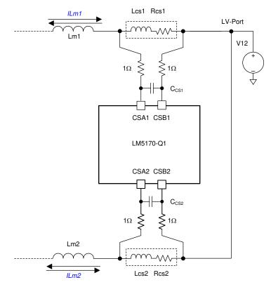
图 9-5. Compensation Network to Compensate the Current Sense Resistor's Parasitic Inductance
