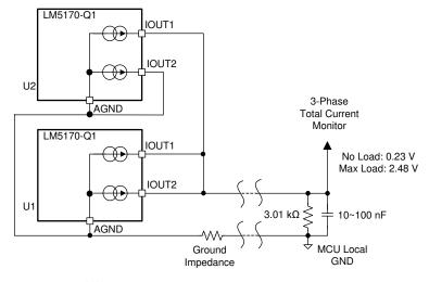
图 8-26. 3-Phase Total Current Monitor
