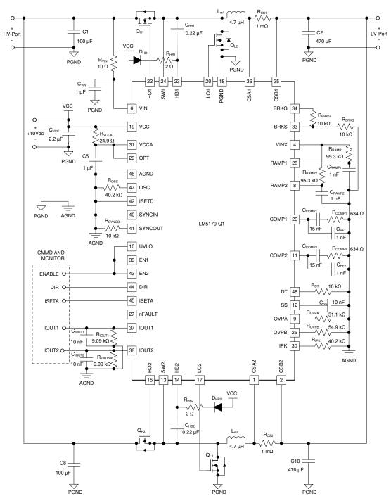
图 9-8. Schematic of the Example Dual-Phase Bidirectional Converter
