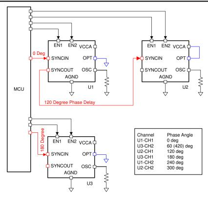
图 8-22. Six Phases 60° Interleaving Configuration
