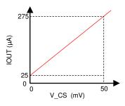
图 8-5. Channel Monitor Current Source vs Current Sense Voltage
