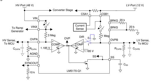
图 8-18. Overvoltage Protection: When Circuit Breaker Function is Not Used
