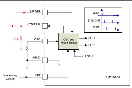
图 8-13. Oscillator and Interleaving Clock Programming
