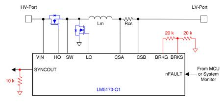
图 8-17. Circuit Breaker Function Disabled
