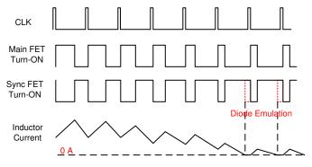
图 8-14. Diode Emulation Operation
