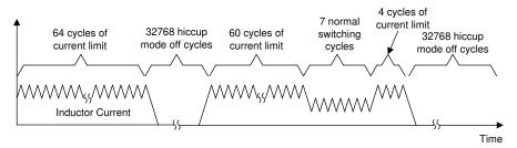
图 9-21. Hiccup Mode Overload Protection
