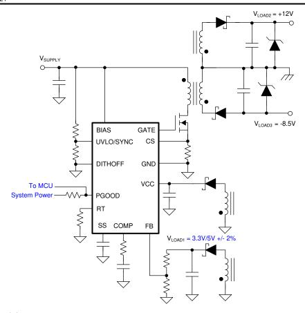
图 10-11. Primary-Side Regulated Multiple-Output Isolated Flyback
