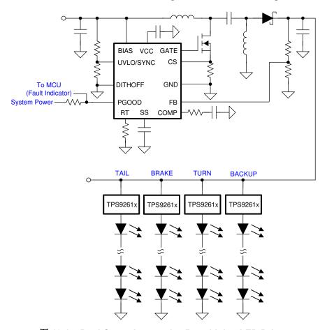
图 10-14. Dual-Stage Automotive Rear-Lights LED Driver
