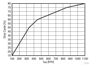
图 9-13. Required Duty Cycle to Start Up by SYNC
