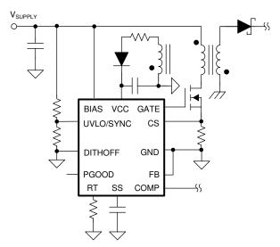
图 9-7. External VCC Supply (BIAS ≥ VCC)
