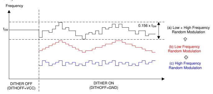
图 9-10. Dual Random Spread Spectrum
