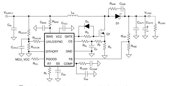
图 10-1. Typical Boost Converter Circuit With Optional Components
