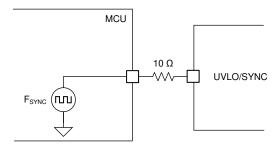
图 9-16. Shutdown and Clock Synchronization
