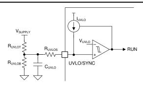
图 9-4. Line UVLO Using Three UVLO Resistors
