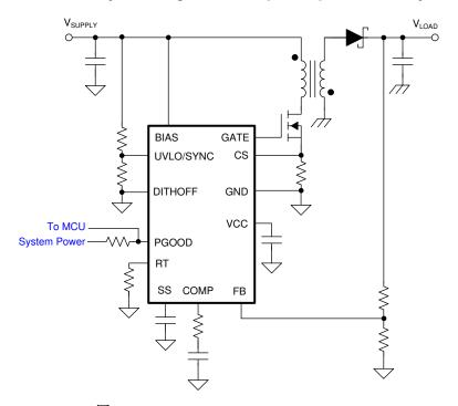
图 10-12. Typical Non-Isolated Flyback
