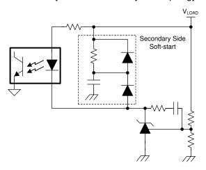
图 9-9. Secondary-Side Soft Start in Flyback
