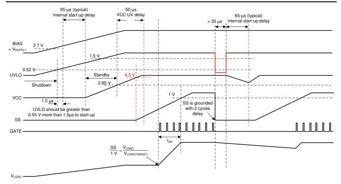
图 9-3. Boost Start-Up Waveforms Case 2: Start-Up When VCC > 4.5 V, EN Toggle After Start-Up
