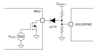
图 9-14. UVLO, Standby, and Clock Synchronization (a)
