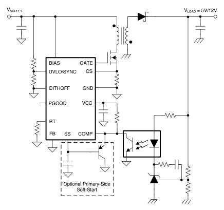
图 10-10. Secondary-Side Regulated Isolated Flyback
