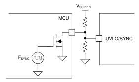
图 9-12. UVLO, Shutdown, and Clock Synchronization
