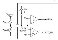
图 9-1. Line UVLO and Enable
