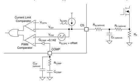
图 9-18. Current Sensing and Slope Compensation
