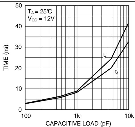
Figure 7. Rise and Fall Time vs Capacitive Load
