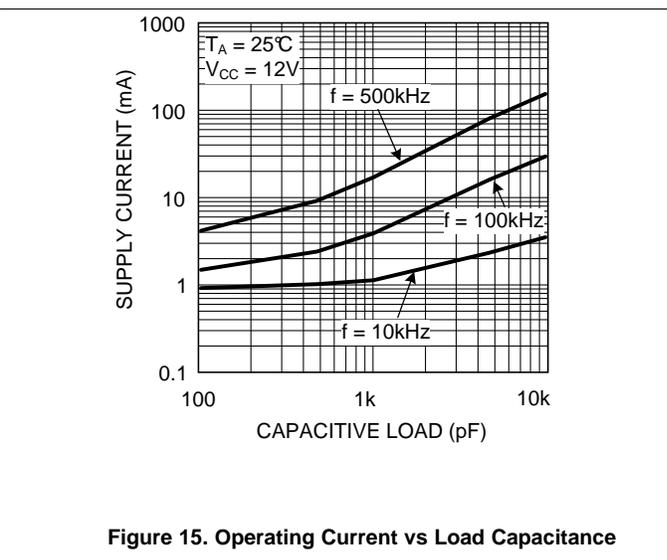
Figure 15. Operating Current vs Load Capacitance
