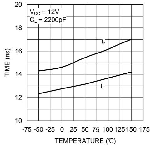
Figure 6. Rise and Fall Time vs Temperature
