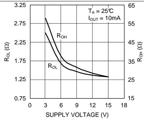
Figure 10. R<sub>DS(on)</sub> vs Supply Voltage
