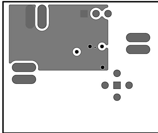
Figure 44. Layer 3 (V<sub>DD</sub>)
