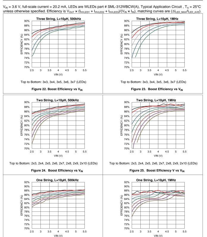
Top to Bottom: 1x3, 1x4, 1x5, 1x6, 1x7, 1x8, 1x9, 1x10 (LEDs)
