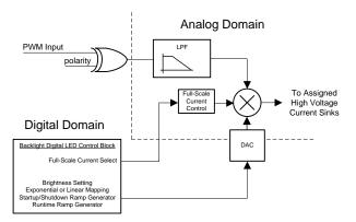
Figure 9. PWM Input Architecture
