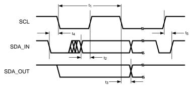
Figure 1. I<sup>2</sup>C-Compatible Interface Timing
