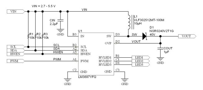
Figure 13. LM3697 Schematic
