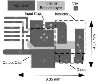
Figure 59. LM3697 Layout Example
