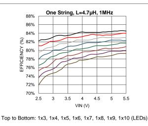
Figure 33. Boost Efficiency vs VIN
