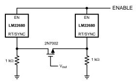
Figure 14. Self Synchronizing Setup
