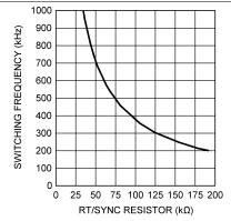
Figure 10. Switching Frequency vs RT/SYNC Resistor
