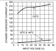
Figure 7. Standby Quiescent Current vs Input Voltage
