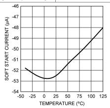
Figure 11. Soft-Start Current vs Temperature
