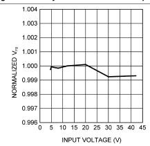
Figure 9. Normalized Feedback Voltage vs Input Voltage
