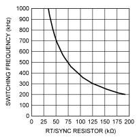
Figure 13. Switching Frequency vs RT/SYNC Resistor
