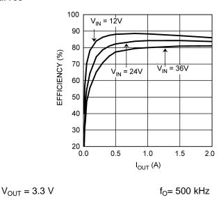
Figure 21. Efficiency vs I<sub>OUT</sub> and V<sub>IN</sub>
