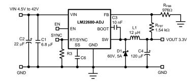
Figure 20. Typical Buck Regulator Application
