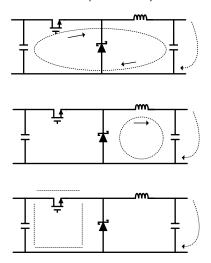
Figure 22. Current Flow in a Buck Application
