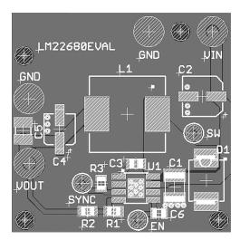
Figure 23. LM2280 Layout Example
