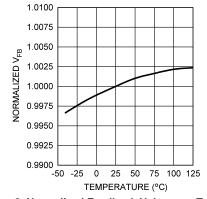
Figure 8. Normalized Feedback Voltage vs Temperature
