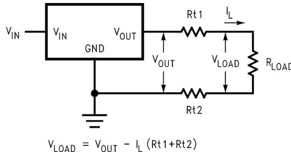
图 6-2. Typical Application Using Fixed Output Regulator
