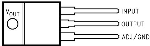
图 4-1. 3-Pin TO-220 Package Top View
