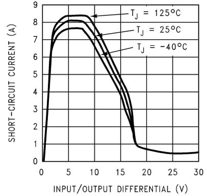
图 5-2. Short-Circuit Current
