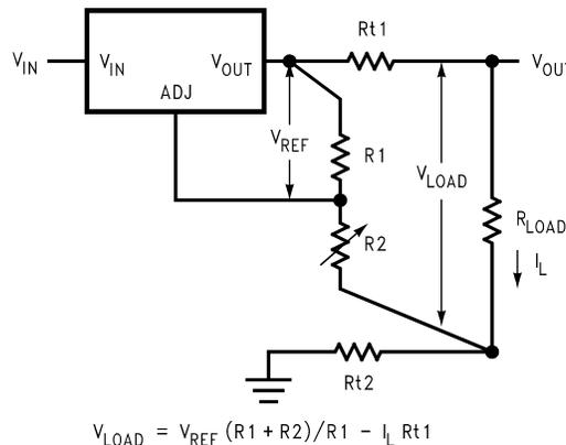
图 6-3. Best Load Regulation Using Adjustable Output Regulator
