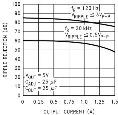
图 5-5. LM1084-ADJ Ripple Rejection vs Current
