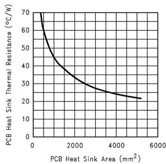
**图 7-14. Heat Sink Thermal Resistance vs Area**
