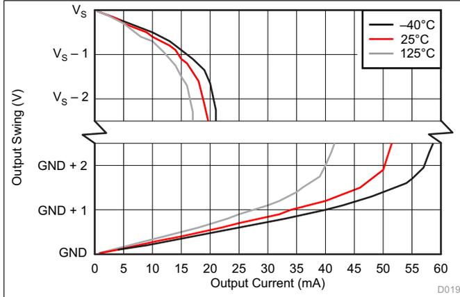
图 19. Output Voltage Swing vs Output Current
