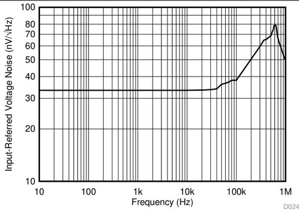
图 25. Input-Referred Voltage Noise vs Frequency (INA381A3 Devices)
