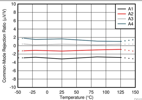
图 10. Common-Mode Rejection Ratio vs Temperature
