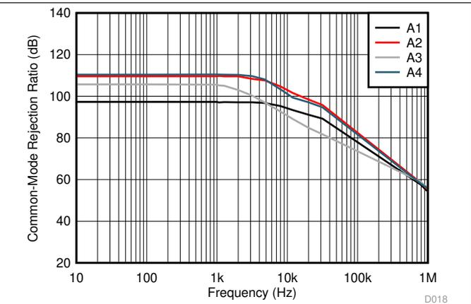
图 18. Common-Mode Rejection Ratio vs Frequency
