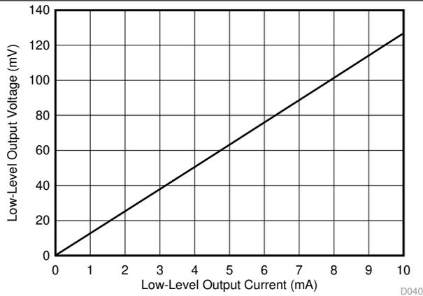
**图 37. Low-Level Output Voltage vs Low-Level Output Current**
