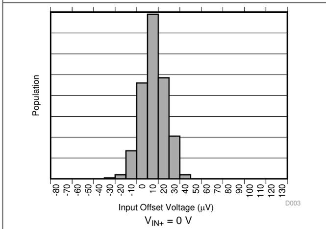
图 3. Input Offset Voltage Production Distribution (INA381A3)
