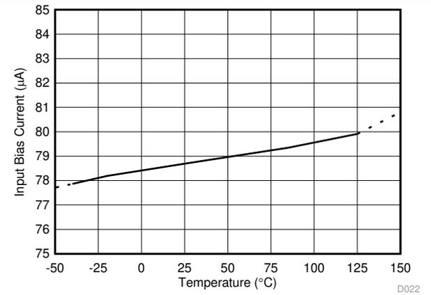
图 22. Input Bias Current vs Temperature
