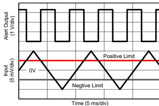
**图 51. Bidirectional Operation**
