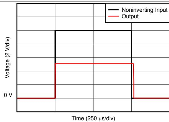
图 30. Noninverting Differential Input Overload
