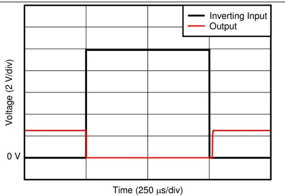
图 29. Inverting Differential Input Overload
