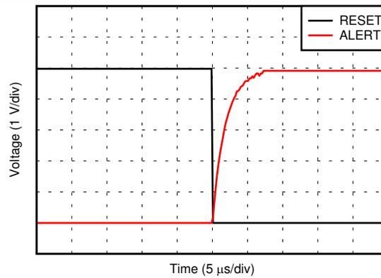
**图 39. Reset and Alert Voltage Response**
