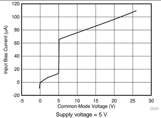
图 20. Input Bias Current vs Common-Mode Voltage
