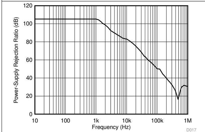
图 17. Power-Supply Rejection Ratio vs Frequency
