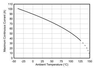
图 8-1. Maximum Continuous Current vs Ambient Temperature
