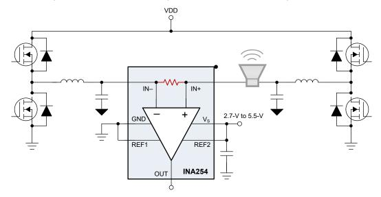
图 9-3. Current Sensing in a CLASS-D Subsystem
