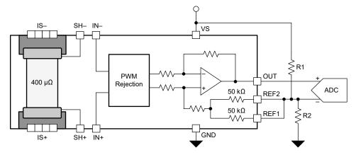
图 8-10. Setting the Reference Using a Resistor Divider
