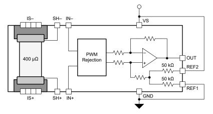
图 8-8. Mid-Supply Voltage Output
