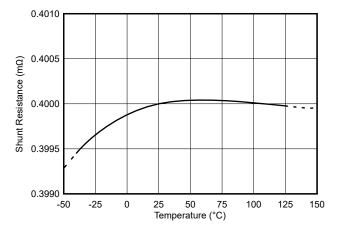
图 8-3. Sensing Resistor vs Temperature
