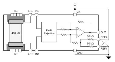
图 8-5. Adjusting the Output Midpoint
