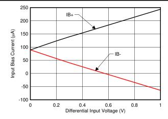
图 9-2. Input Bias Current vs Differential Input Voltage
