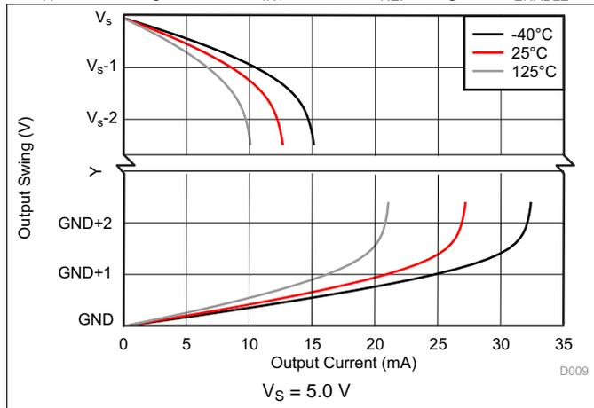
图 13. Output Voltage Swing vs Output Current
