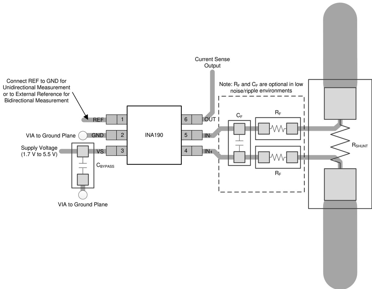
图 46. Recommended Layout for SC70 (DCK) Package
