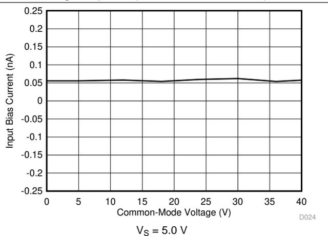
图 14. Input Bias Current vs Common-Mode Voltage
