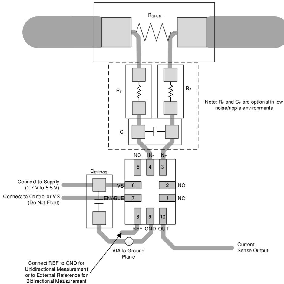
图 48. Recommended Layout for UQFN (RSW) Package
