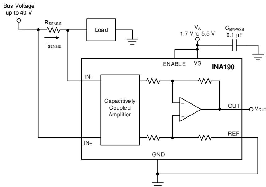
**图 35. Typical Unidirectional Application**
