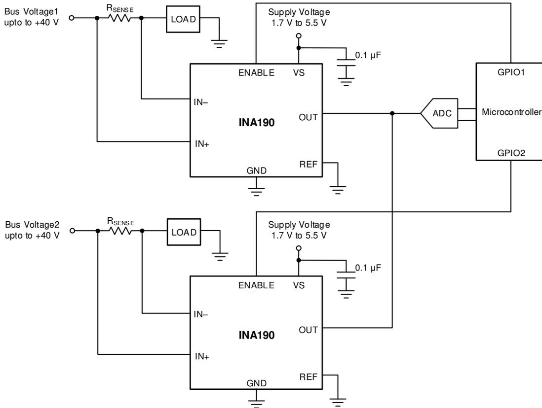
图 38. Multiplexing Multiple Devices With the ENABLE Pin
