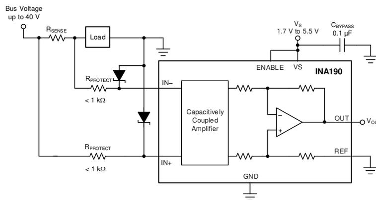
图 42. Transient Protection Using Dual Zener Diodes
