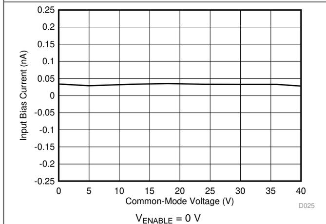
图 15. Input Bias Current vs Common-Mode Voltage (Shutdown)
