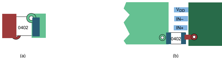
图 21. Typical Decoupling Capacitor Layouts
