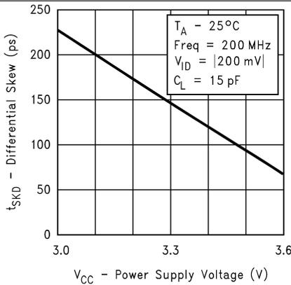
Figure 9. Differential Skew vs Power Supply Voltage
