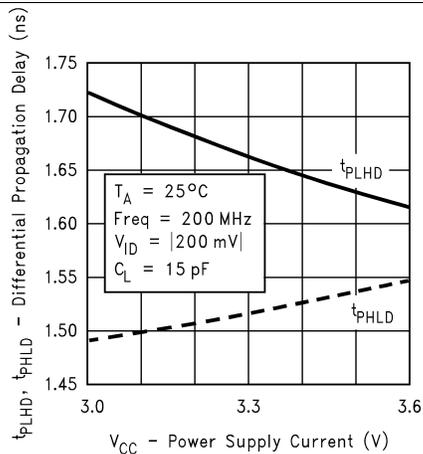
**Figure 5. Differential Propagation Delay vs Power Supply Voltage**
