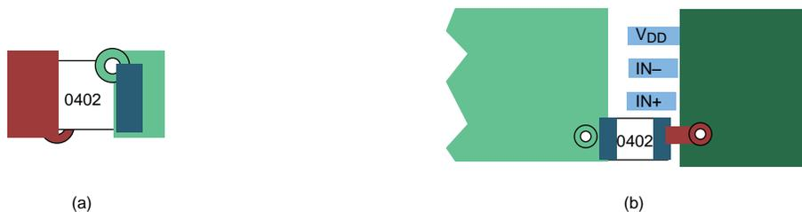
Figure 27. Typical Decoupling Capacitor Layouts
