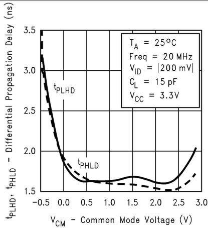
Figure 7. Differential Propagation Delay vs Common-Mode Voltage
