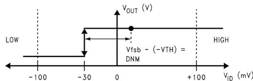
**Figure 16. VTC of the DS90LV028AH LVDS Receiver**
