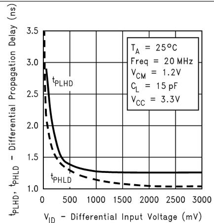
**Figure 6. Differential Propagation Delay vs Differential Input Voltage**
