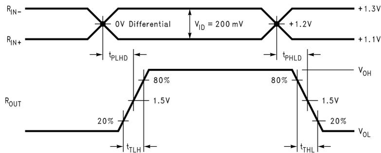
Figure 15. Receiver Propagation Delay and Transition Time Waveforms
