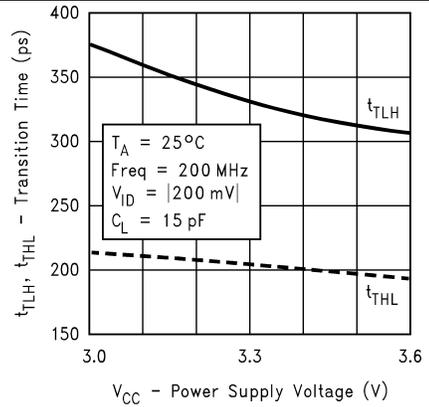
Figure 8. Transition Time vs Power Supply Voltage
