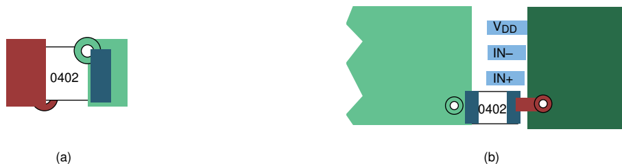
图 11-7. Typical Decoupling Capacitor Layouts
