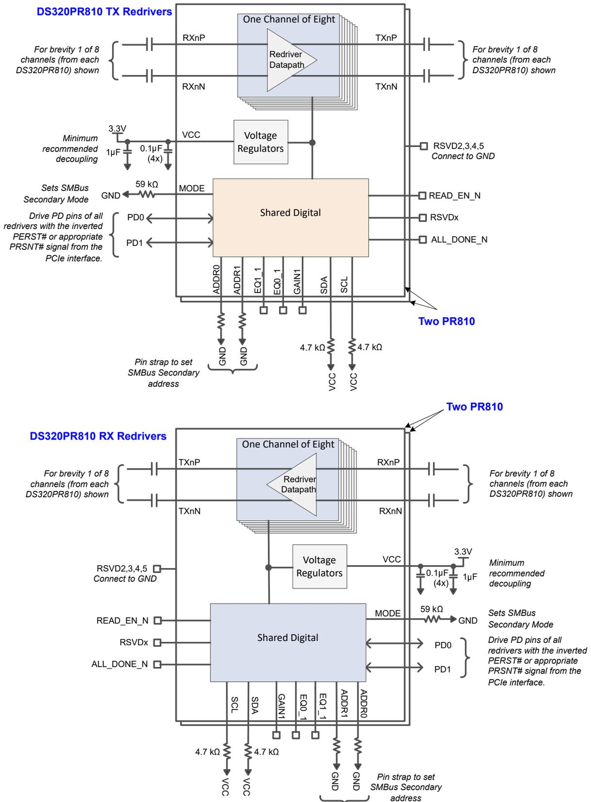
图 8-4. Simplified Schematic for PCIe x16 Lane Configuration in SMBus/I<sup>2</sup>C Secondary mode
