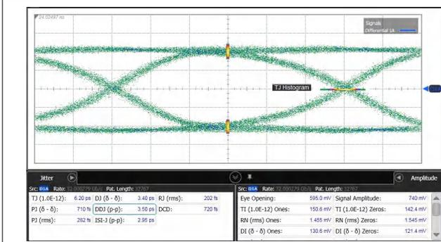
图 6-4. At BERT Source Output (1 dB Loss)
