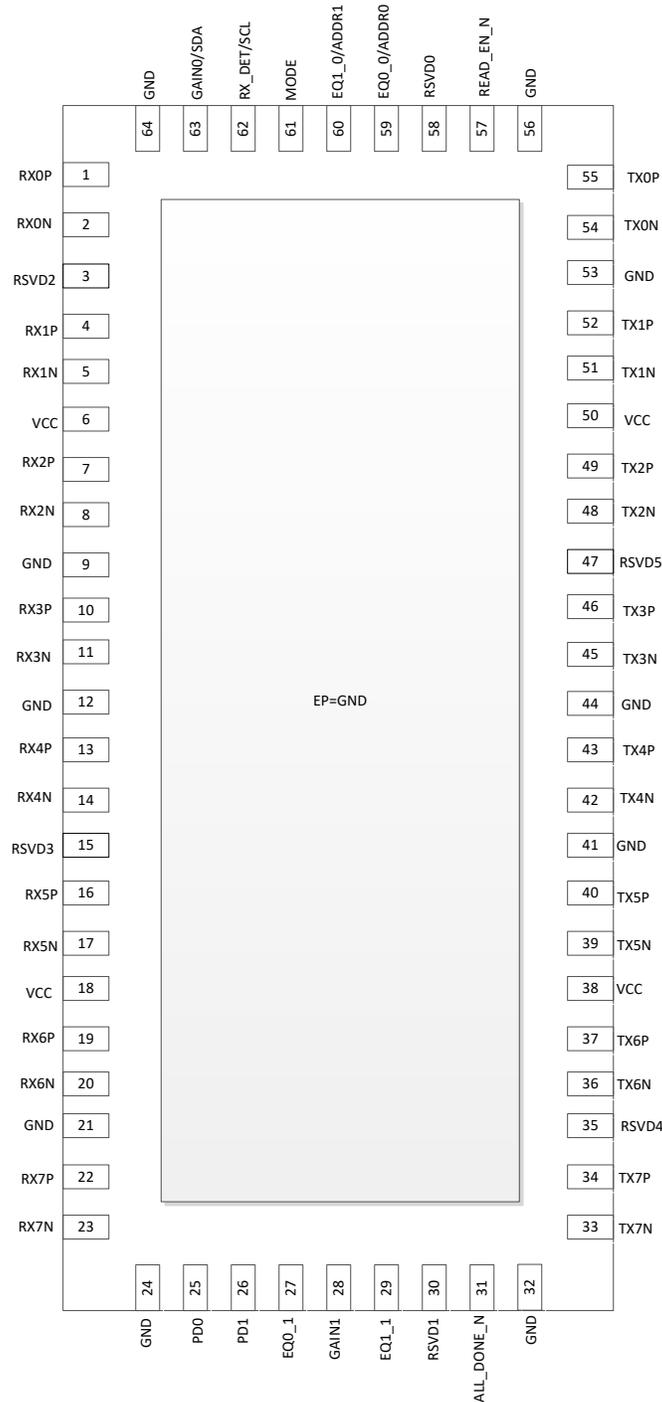
图 5-1. NJX Package, 64-Pin WQFN (Top View)
