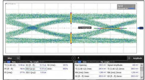
图 6-5. Through Baseline Calibration Trace Setup (7 dB Loss)
