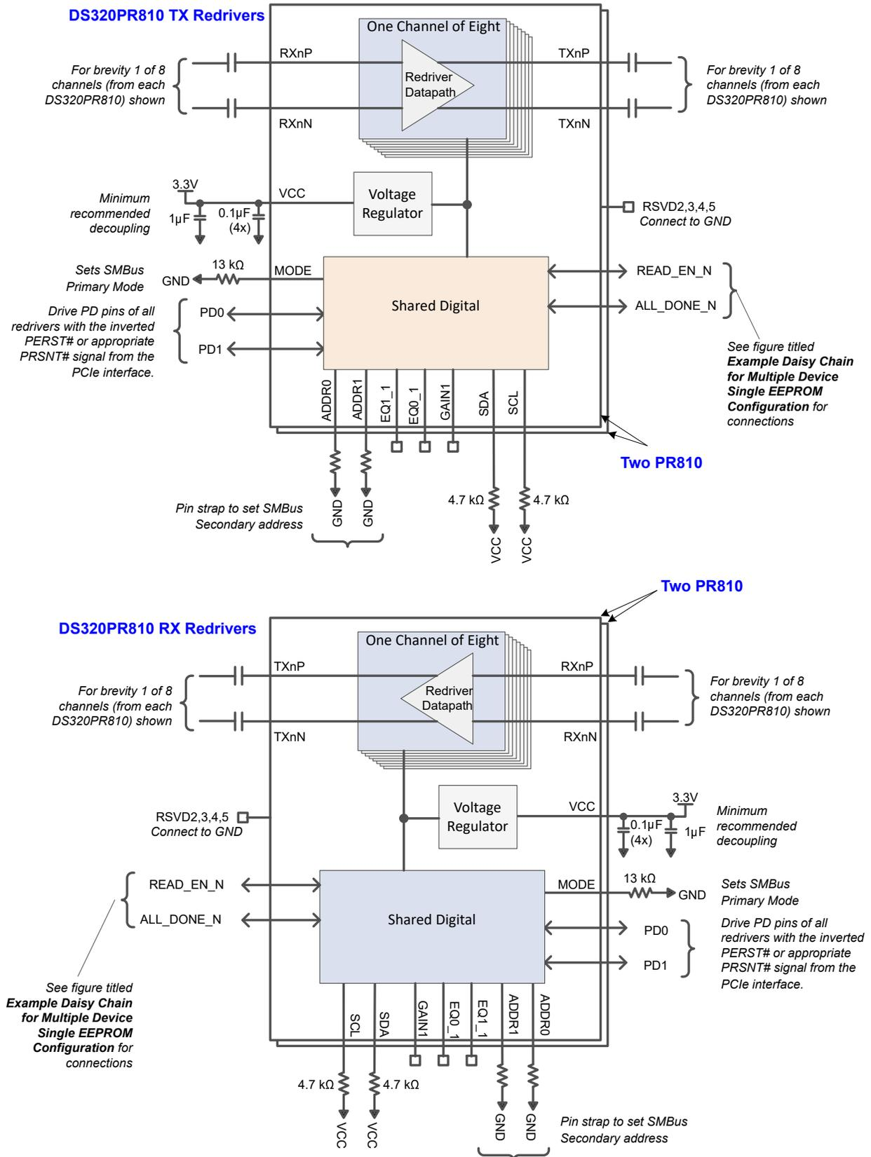
图 8-3. Simplified Schematic for PCIe x16 Lane Configuration in SMBus/I<sup>2</sup>C Primary mode
