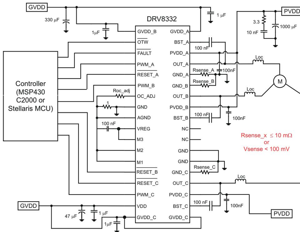
图 8-1. DRV8332 Application Diagram for Three-Phase Operation Schematic
