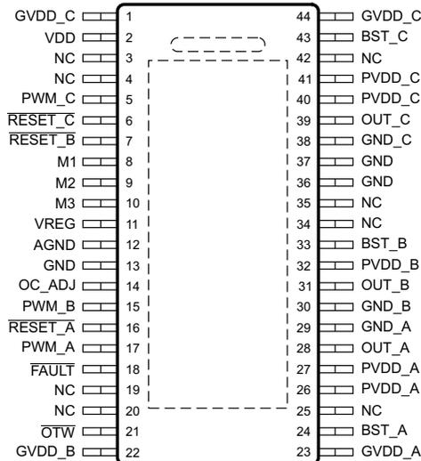
DRV8312: 44-pin TSSOP power pad down DDW package. This package contains a thermal pad that is located on the bottom side of the device for dissipating heat through PCB.
