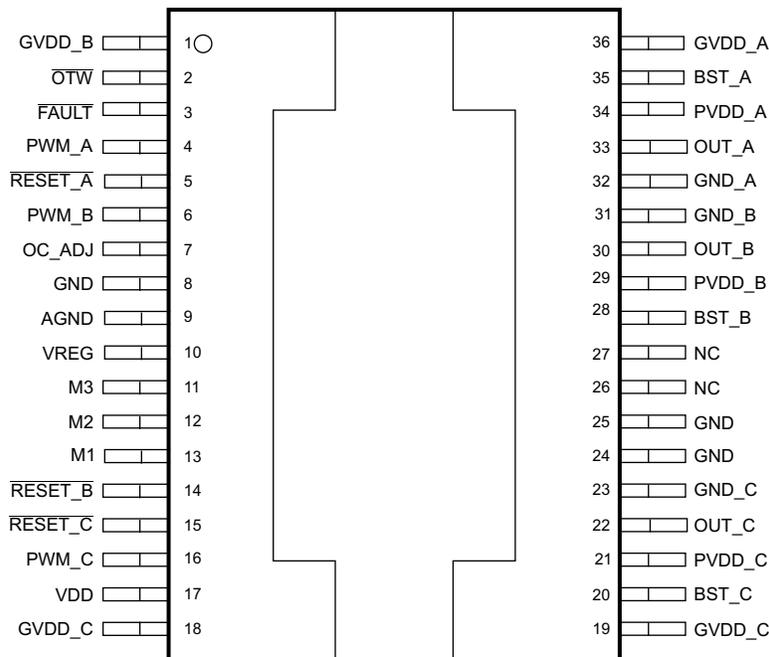
DRV8332: 36-pin PSOP3 DKD package. This package contains a thick heat slug that is located on the top side of the device for dissipating heat through heatsink.
