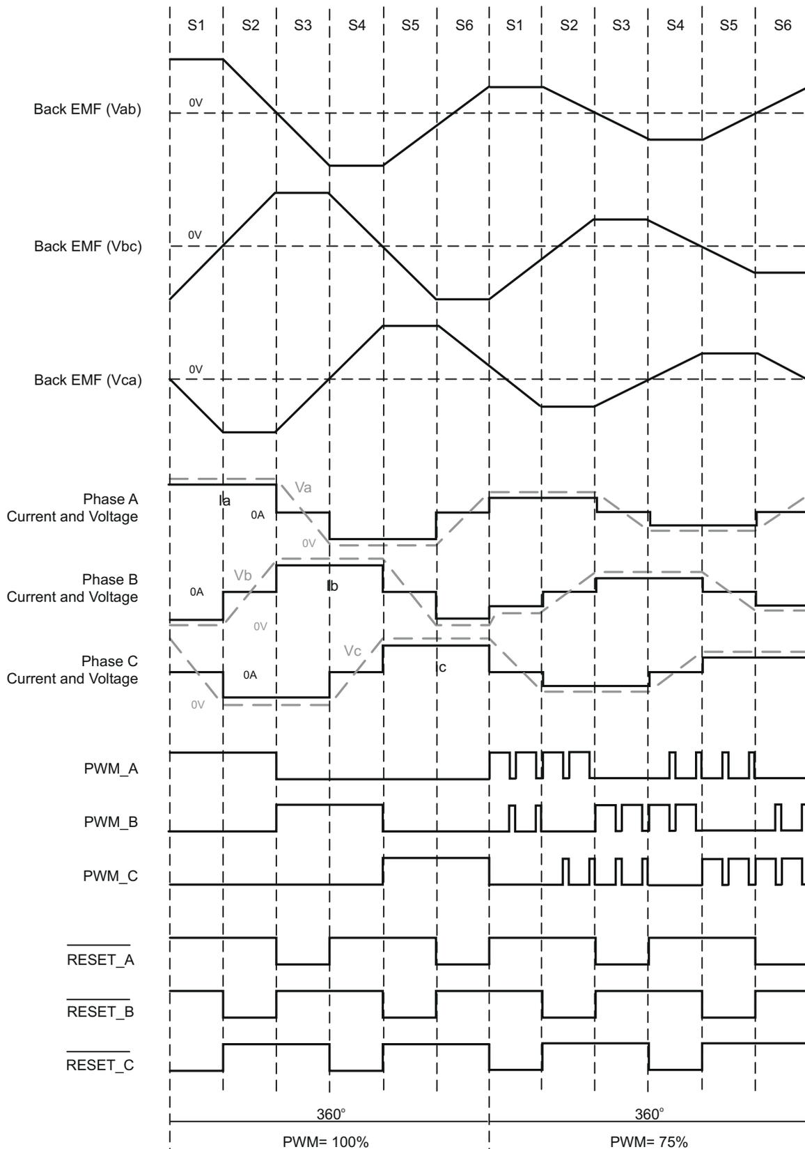
图 8-7. Sensorless Control With 6 Steps Trapezoidal Scheme Schematic
