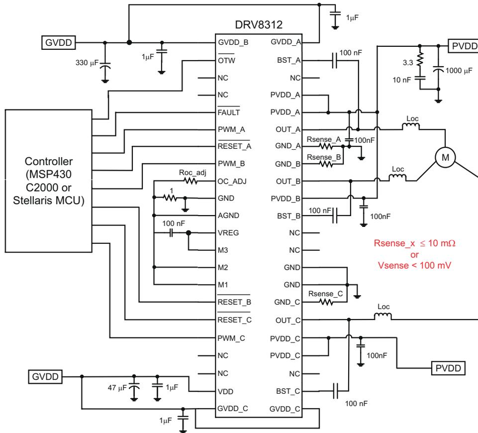
图 8-4. DRV8312 Application Diagram for Three-Phase Operation Schematic
