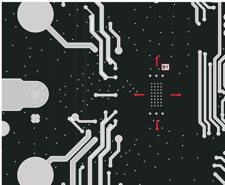
B1: Do not block the heat transfer path at bottom side. Clear as much space as possible for better heat spreading.
