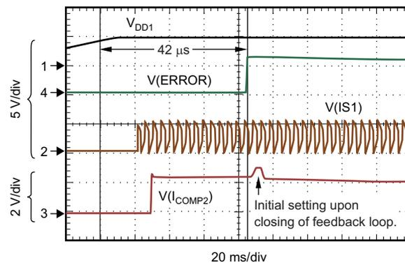
The probe oscillation  $V(IS1)$  starts just before ERROR resets—15  $\mu s$  after the supply voltage crosses the 4-V threshold.
