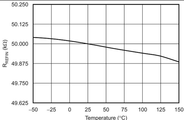
图 19. Differential Amplifier: REF<sub>IN</sub> Resistance vs Temperature
