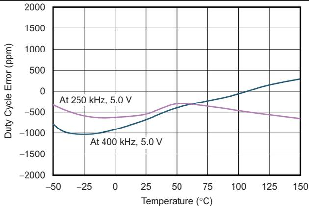
图 21. Compensation Loop: Duty Cycle Error vs Temperature
