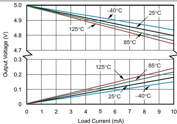
图 10. Differential Amplifier: Output Voltage vs Output Current
