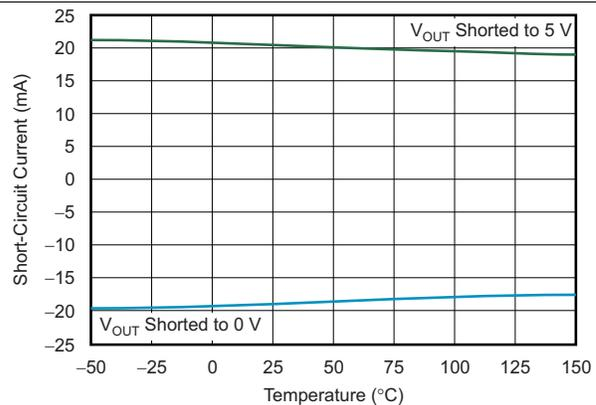
图 12. Differential Amplifier: Short-Circuit Current vs Temperature
