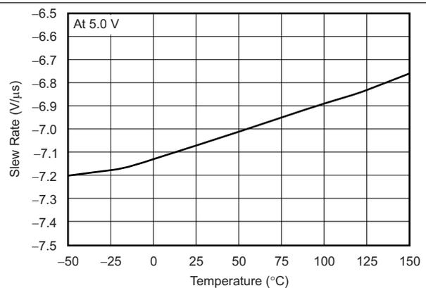
图 18. Differential Amplifier: Negative Slew Rate vs Temperature
