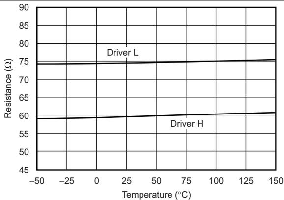
图 25. Probe Driver: Internal Resistor vs Temperature
