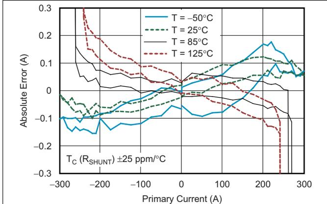
图 3. DRV401-Q1 Device and Sensor: Absolute Error
