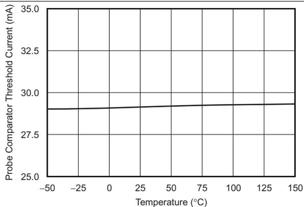
图 24. Probe Comparator Threshold Current vs Temperature
