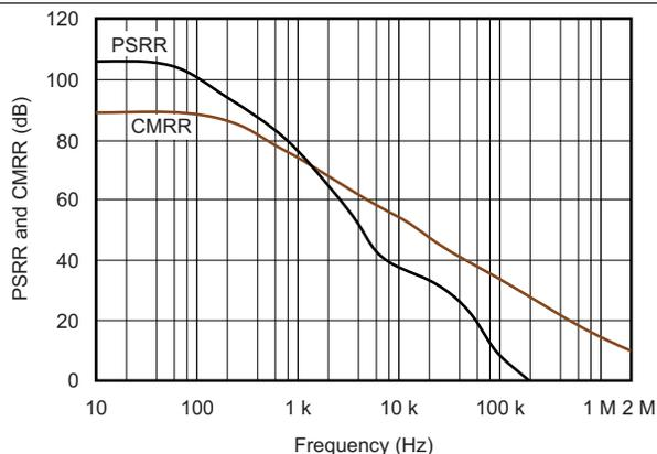
图 9. Differential Amplifier: PSRR and CMRR vs Frequency
