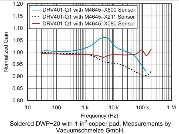
图 4. Gain Flatness vs Frequency
