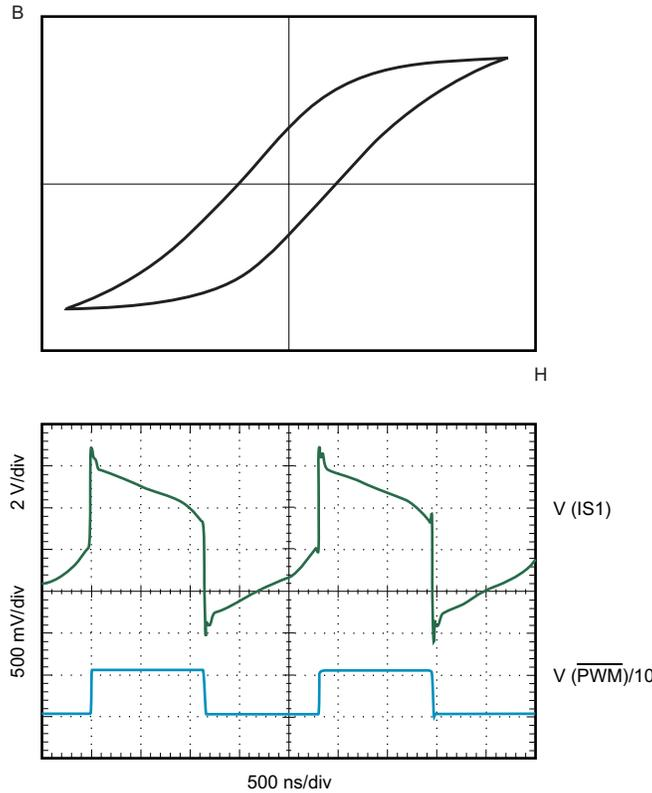
Without an external magnetic field, the hysteresis curve is symmetrical and the probe loop generates 50% duty cycle.
