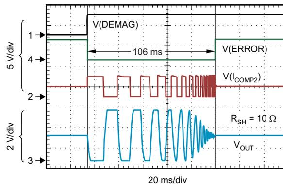
图 48. Demagnetization and Power-On Timing: Demagnetization Cycle On Command
