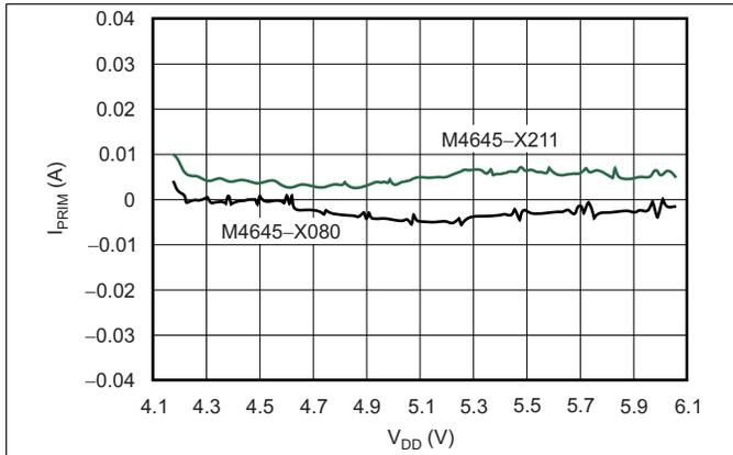
图 1. DRV401-Q1 Device and Sensor: Offset vs Supply Voltage
