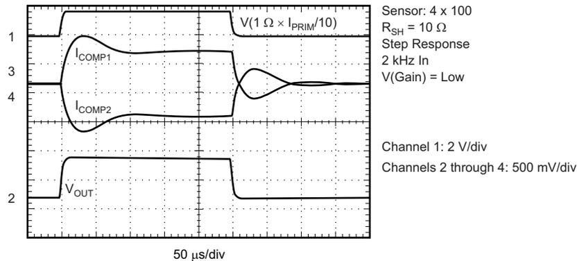
A current pulse of 0 A to 18 A (channel 1) generates the two  $I_{COMP}$  signals (channel 3 and channel 4). Channel 2 shows the resulting output signal ( $V_{OUT}$ ). This test uses the M4645-X030 sensor with no bandwidth limitation, and a 20-sample average.
