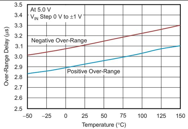
图 16. Differential Amplifier: Overrange Delay vs Temperature
