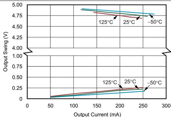
图 23. I<sub>COMP</sub> Output Swing to Rail vs Output Current
