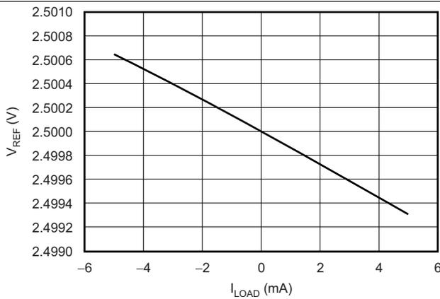
图 27. Voltage Reference vs Load Current
