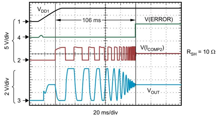
With power-up, the  $V_{OUT}$  across the compensation coil centers around half the supply and then starts the cycle after the 4-V threshold is exceeded. The ERROR flag resets to H after the cycle is completed.
