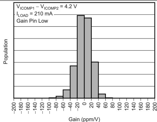
图 22. Compensation Loop: DC Gain: Duty Cycle Error Change
