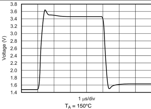
图 15. Differential Amplifier: Large-Signal Step Response
