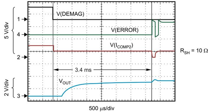
The ERROR flag resets to H (as shown) and the output settles back to normal operation.
