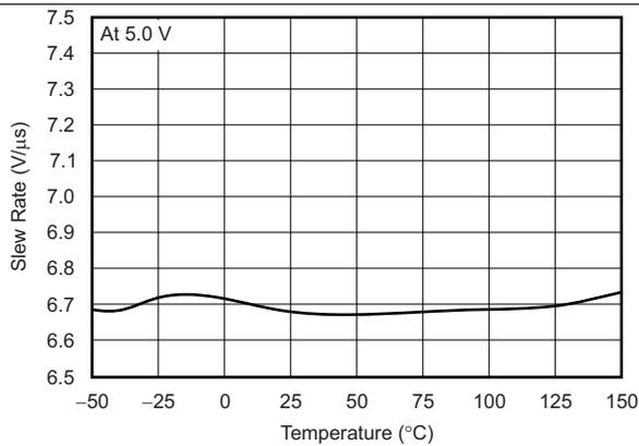
图 17. Differential Amplifier: Positive Slew Rate vs Temperature
