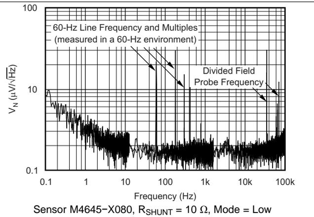
图 2. DRV401-Q1 Device and Sensor: Output Voltage Noise Density
