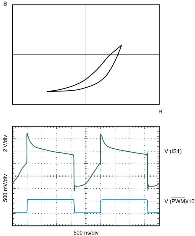
An external magnetic flux (H) generated from the primary current ( $I_{PRIM}$ ) shifts the hysteresis curve of the magnetic field probe in the H-axis and the probe loop generates a nonsymmetrical duty cycle.
