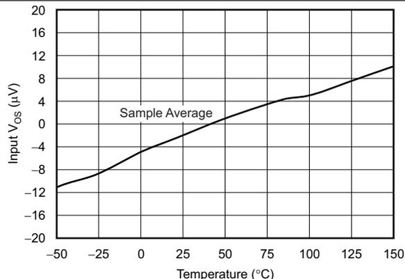
图 7. Differential Amplifier: Offset Voltage vs Temperature, RTO
