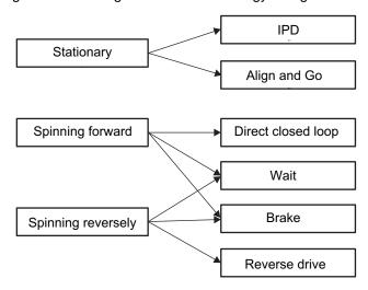
图 10. Start the Motor Under Different Initial Conditions
