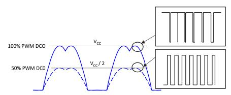
图 7. Output Voltage Amplitude Adjustment
