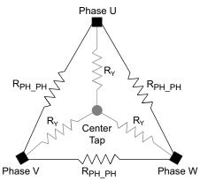
图 9. Delta-Connected Motor and the Equivalent Wye Connections
