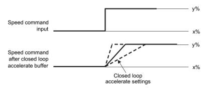
图 25. Closed-Loop Accelerate
