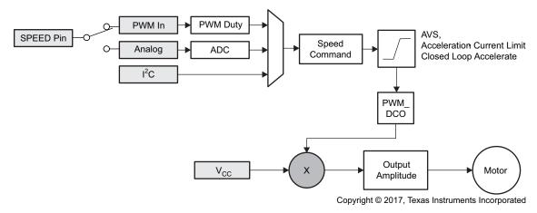
图 4. Multiplexing the Speed Command to the Output Amplitude Applied to the Motor
