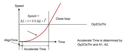
图 18. Motor Start-Up Process
