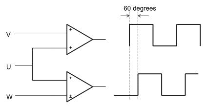
图 12. Initial Speed Detect Function
