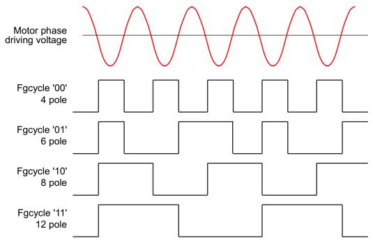
图 35. FG Frequency Divider
