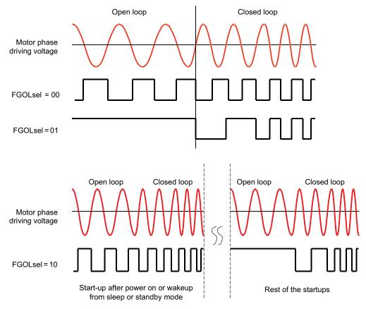
图 36. FG Behavior During Open Loop
