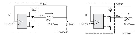
Step-Down Regulator With External Inductor (Buck Mode)
