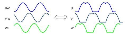
Sinusoidal voltage from phase to phase
