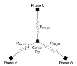
图 8. Wye-Connected Motor Phase Resistance
