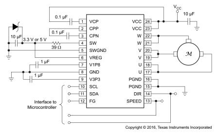
图 39. Typical Application Schematics for DRV10975 (Top Image) and DRV10975Z (Bottom Image)
