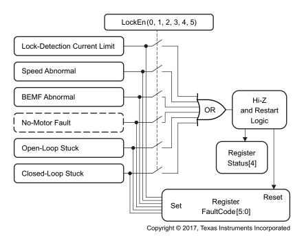
图 28. Lock Detect and Fault Diagnose
