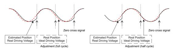
图 21. Closed Loop Control Commutation Adjustment Mode
