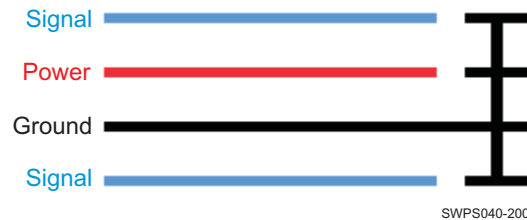
图 7-19. Guard Ring Routing
