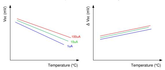
图 7-3. Example of Delta VBE Versus Temperature
