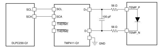
图 7-1. Temperature Sense Diode Typical Circuit Configuration
