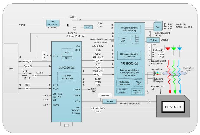
图 8-1. Window Display System Block Diagram
