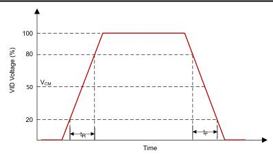
图 6-3. SubLVDS Input Rise and Fall Slew Rate
