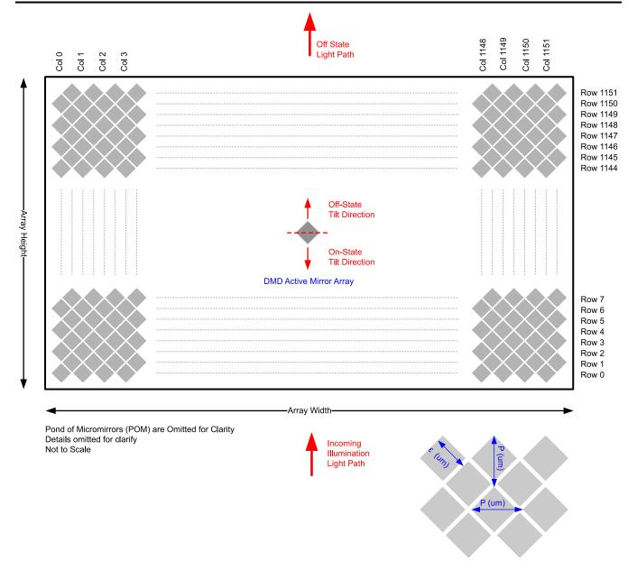
图 6-13. Micromirror Array Physical Characteristics
