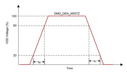
图 6-2. LPSDR Input Rise and Fall Slew Rate
