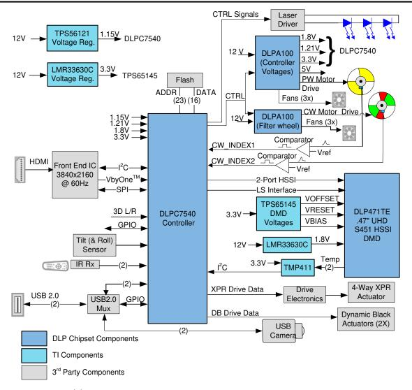
图 8-1. Typical 4K UHD Laser Phosphor Application Diagram
