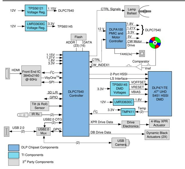
图 8-2. Typical 4K UHD Lamp Application Diagram
