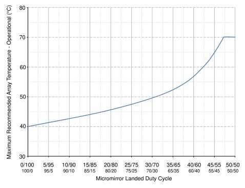
图 6-1. Maximum Recommended Array Temperature—Derating Curve
