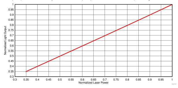
图 8-3. Normalized Light Output vs. Normalized Laser Power for Laser Phosphor Illumination
