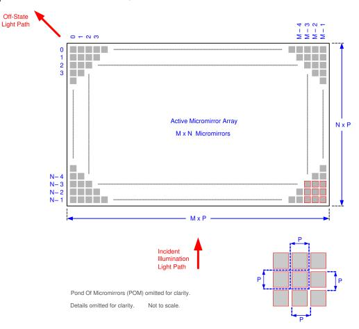
图 6-14. Micromirror Array Physical Characteristics
