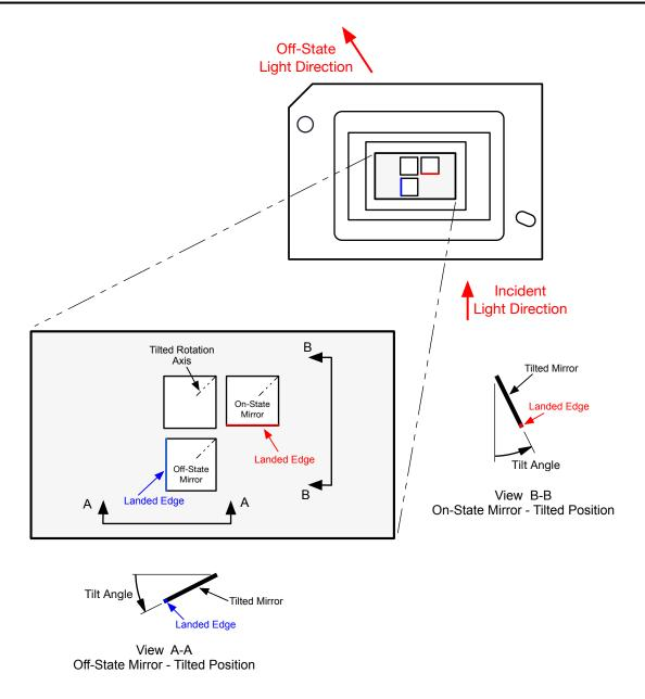
图 6-15. Micromirror Landed Orientation and Tilt
