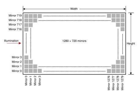
图 6-16. Micromirror Array Physical Characteristics
