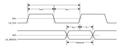
Low-speed interface is LPSDR and adheres to the #6.6 and AC/DC Operating Conditions table in JEDEC Standard No. 209B, Low Power Double Data Rate (LPDDR) JESD209B.
