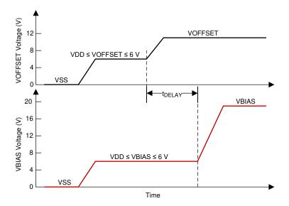
A. Refer to 表 9-1 for  $V_{\sf OFFSET}$  and  $V_{\sf BIAS}$  supply voltage levels during power-up sequence delay.
