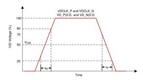
图 6-5. SubLVDS Input Rise and Fall Slew Rate
