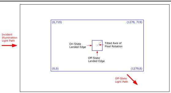
图 6-18. Landed Pixel Orientation and Tilt
