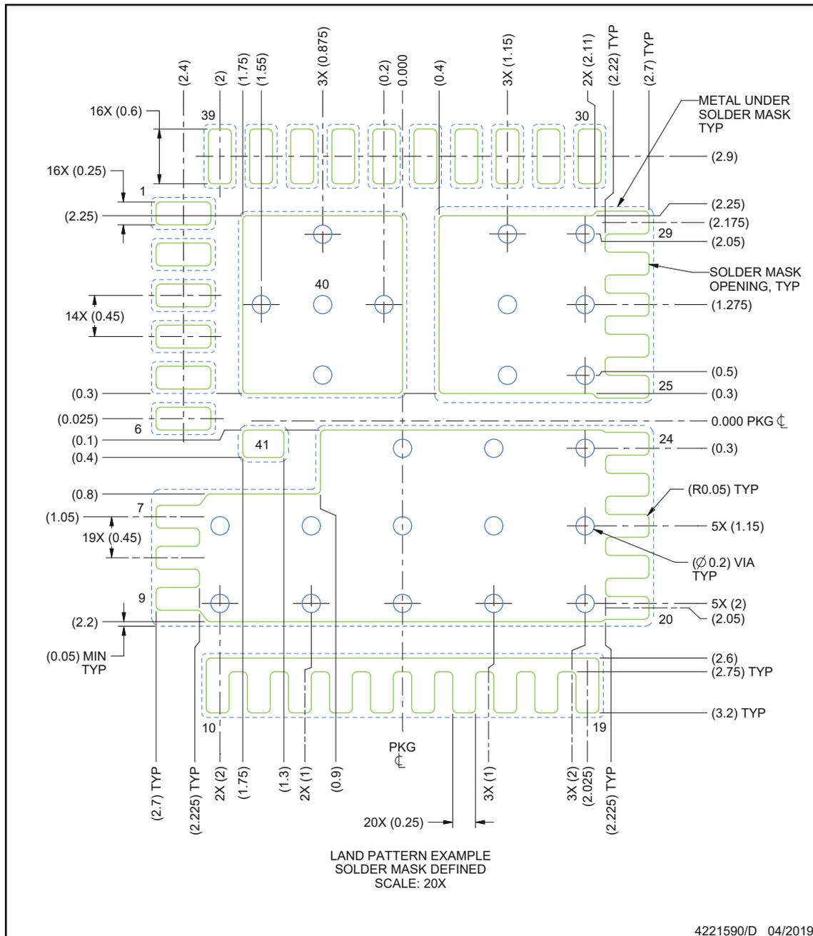
1. All linear dimensions are in millimeters. Any dimensions in parenthesis are for reference only. Dimensioning and tolerancing per ASME Y14.5M.
