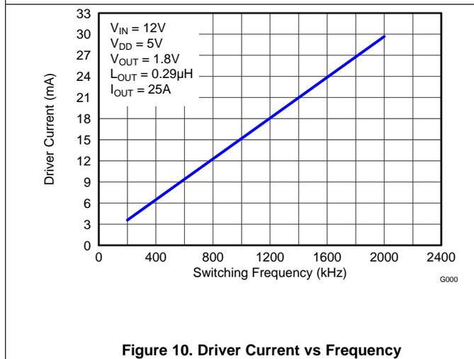
Figure 10. Driver Current vs Frequency
