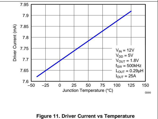
Figure 11. Driver Current vs Temperature
