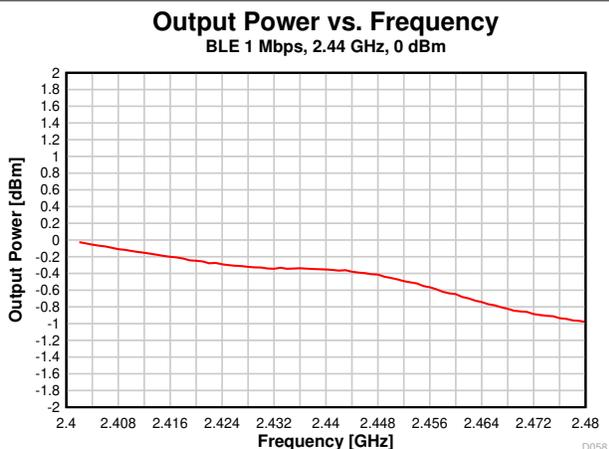
**8-21. Output Power vs. Frequency (BLE 1 Mbps, 2.44 GHz)**
