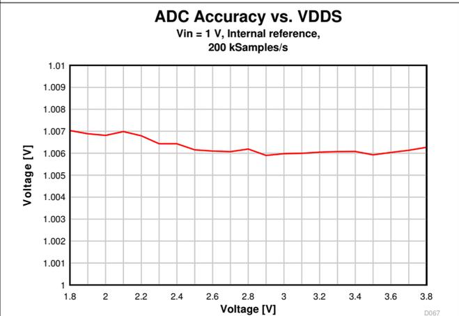
图 8-28. ADC Accuracy vs. Supply Voltage (VDDS)
