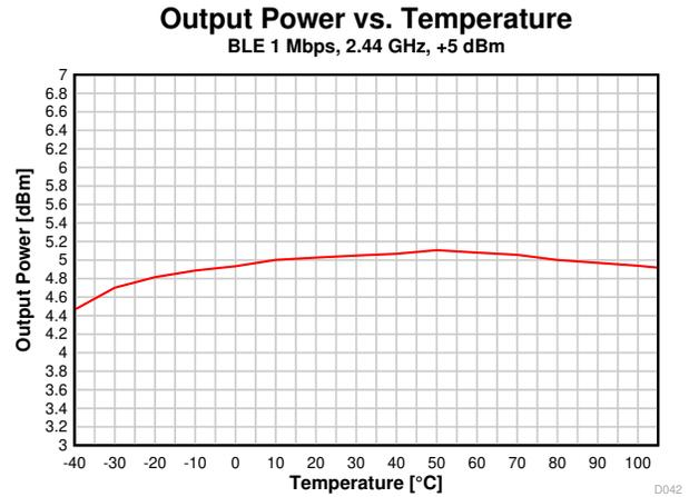
**8-18. Output Power vs. Temperature (BLE 1 Mbps, 2.44 GHz, +5 dBm)**
