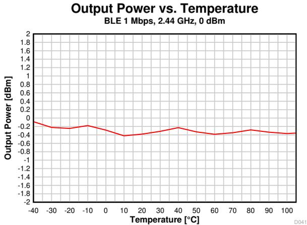
**8-17. Output Power vs. Temperature (BLE 1 Mbps, 2.44 GHz)**
