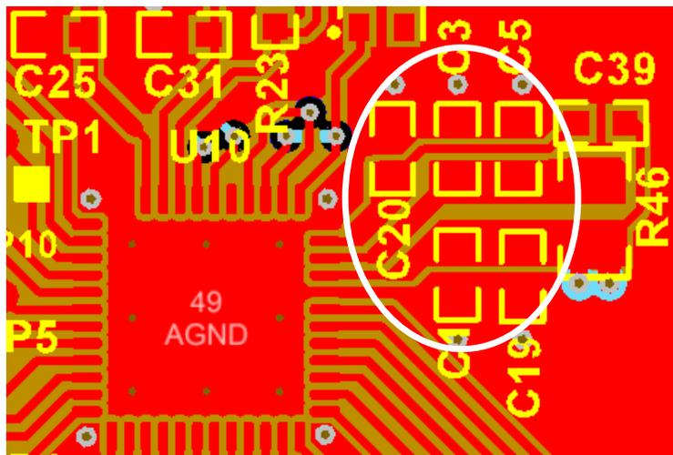
**图 15. Bypass Capacitors Layout**
