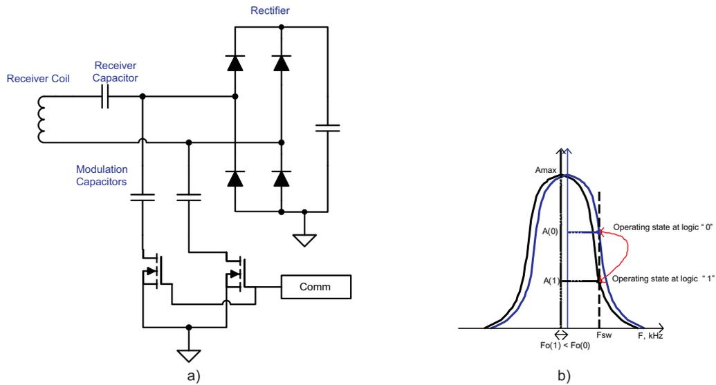
**图 8. Receiver Capacitive Modulation Circuit**
