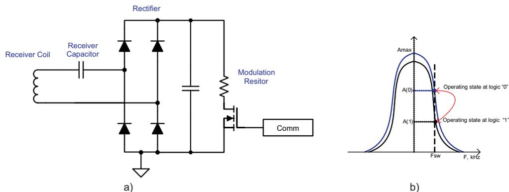
图 7. Receiver Resistive Modulation Circuit
