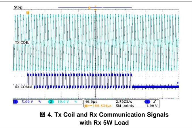
图 4. Tx Coil and Rx Communication Signals with Rx 5W Load
