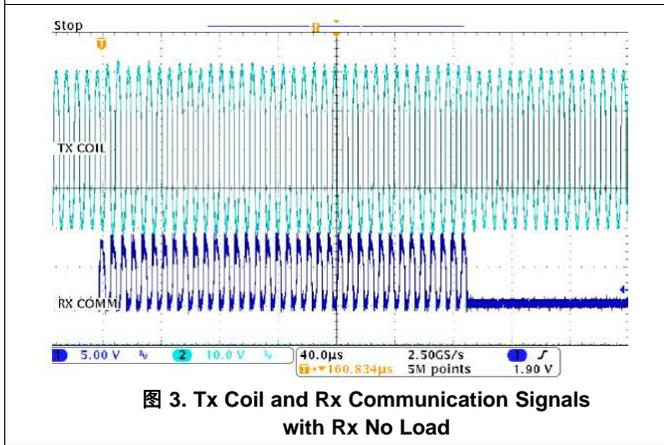
图 3. Tx Coil and Rx Communication Signals with Rx No Load
