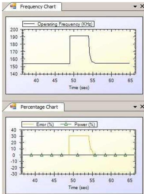
图 11. Qi Sniffer Capture of Frequency Shift Operation
