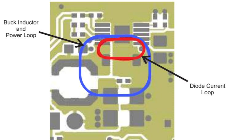
**图 14. DC-DC Buck Regulator Layout**
