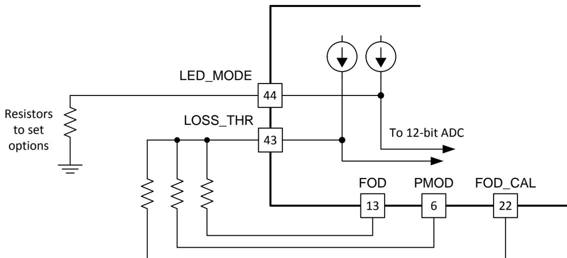
图 5. Pin 43 LOSS\_THR and Pin 44 LED\_MODE Connections
