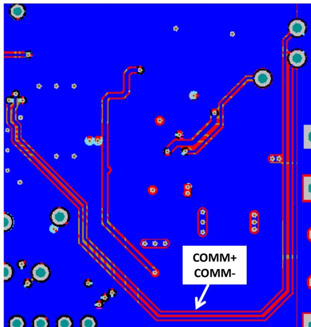
**图 18. Balanced COMM Lines Layout**
