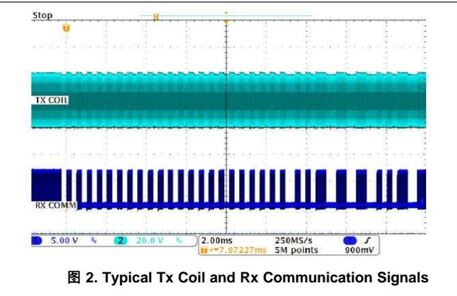
图 2. Typical Tx Coil and Rx Communication Signals
