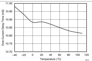
图 14. Overcurrent Delay Time vs. Temperature
