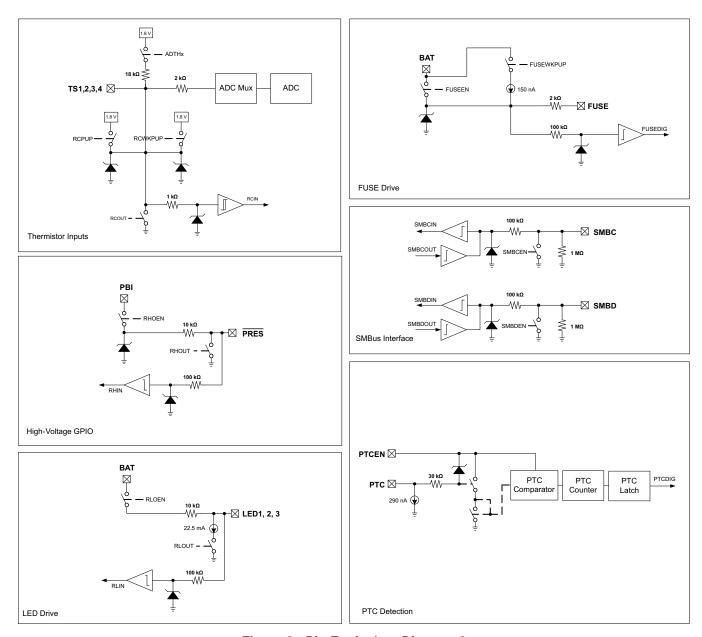
Figure 2. Pin Equivalent Diagram 2
