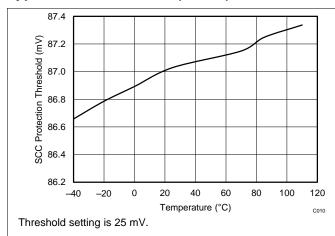
图 11. Short Circuit Charge Protection Threshold vs.
