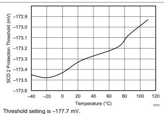
图 13. Short Circuit Discharge 2 Protection Threshold vs.
