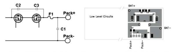
图 47. Use Wide Copper Traces to Lower the Inductance of Bypass Capacitors C1, C2, and C3
