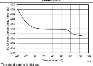
图 15. Short Circuit Charge Current Delay Time vs. Temperature
