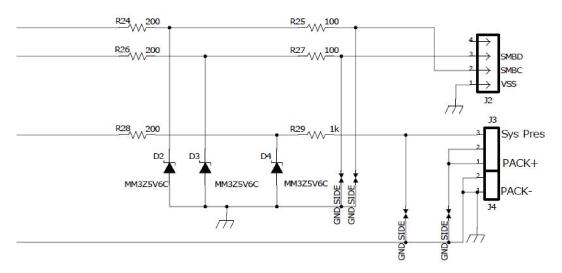
图 30. ESD Protection for SMB Communication
