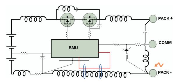
图 44. Avoid Close Spacing Between High-Current and Low-Level Signal Lines
