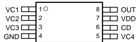
DCT PACKAGE (TOP VIEW)
