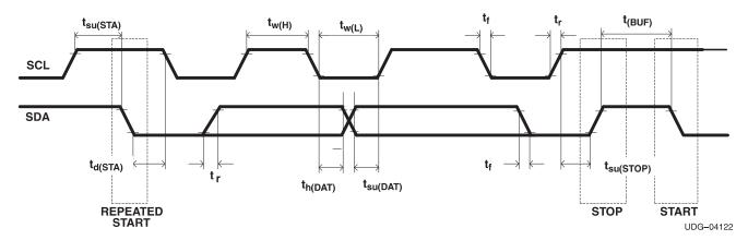
Figure 3-1. I<sup>2</sup>C-Compatible Interface Timing Diagrams
