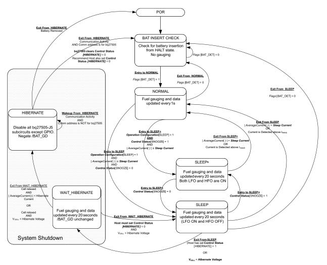
Figure 5-1. Power Mode Diagram
