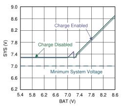
图 19. System Voltage vs. Battery Voltage
