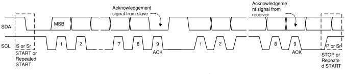
图 29. Data Transfer on the I<sup>2</sup>C Bus
