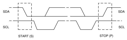
图 28. START and STOP Conditions on the  $I^2C$  Bus
