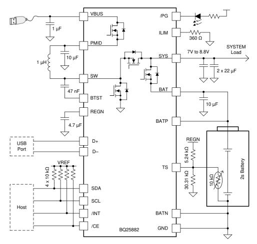
图 75. BQ25882 Typical Application Diagram
