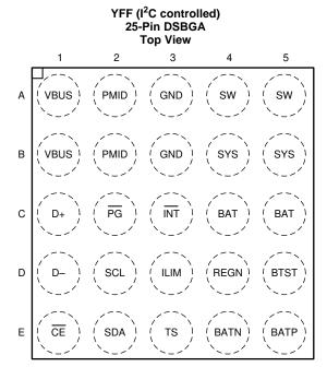
Top View = Xray through a soldered down part with A1 starting in upper left corner
