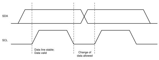
图 27. Bit Transfers on the I<sup>2</sup>C bus
