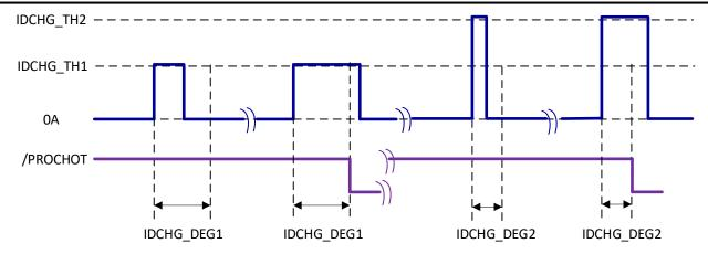
图 8-1. Two-Level Battery Discharging Current Trigger PROCHOT Diagram
