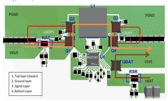
图 11-1. Buck-Boost Charger Layout Reference Example Top View
