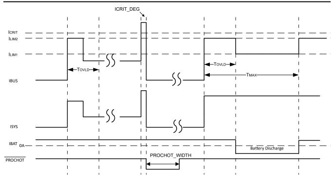
图 8-3. Two-Level Adapter Current Limit Timing Diagram
