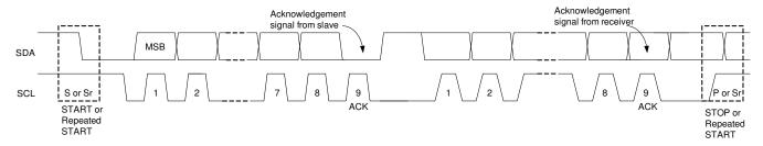
图 8-10. Data Transfer on the I<sup>2</sup>C Bus
