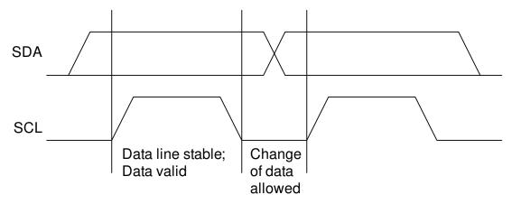
图 8-8. Bit Transfer on the I<sup>2</sup>C Bus
