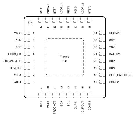
图 6-1. RSN Package 32-Pin WQFN Top View
