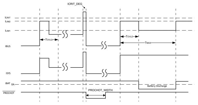
图 9-3. Two-Level Adapter Current Limit Timing Diagram
