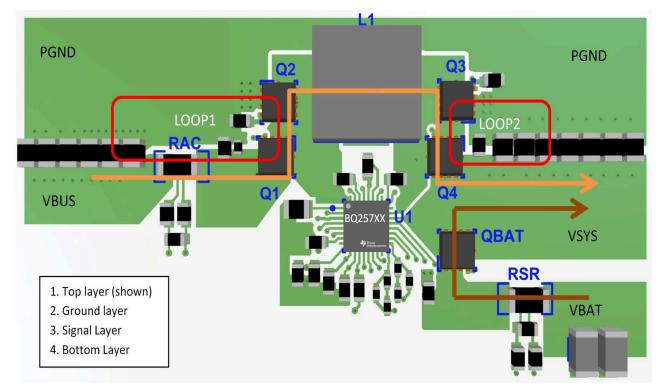
图 12-1. Buck-Boost Charger Layout Reference Example Top View
