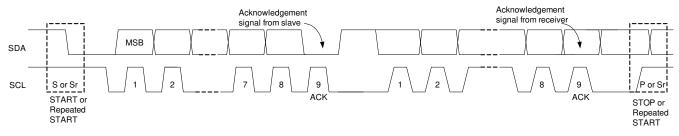
图 9-10. Data Transfer on the I<sup>2</sup>C Bus
