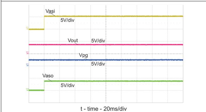
**图 9-4. - ASI and OUT Power-up Timing - No Input**
