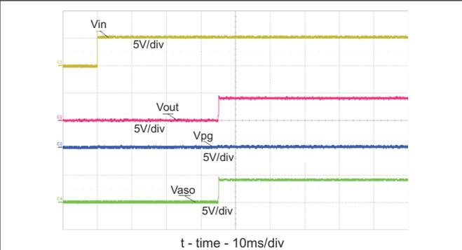
**图 9-3. Power-up Timing - No Battery or Load**
