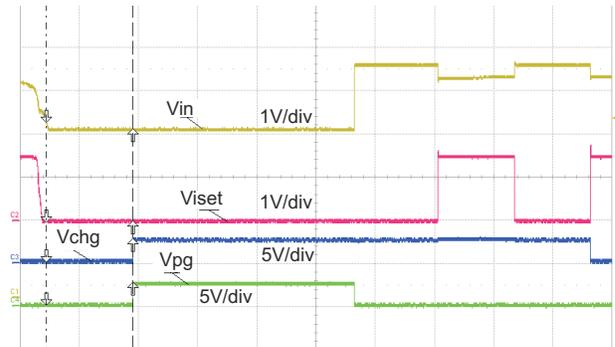
V<sub>IN</sub> swept from 5V to 3.9V to 5V
