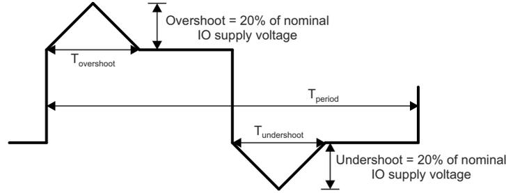
A.  $T_{\text{overshoot}} + T_{\text{undershoot}} < T_{\text{period}}$  的 20%
