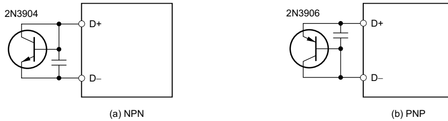
图 7-6. Remote Temperature Sensor Using Transistor
