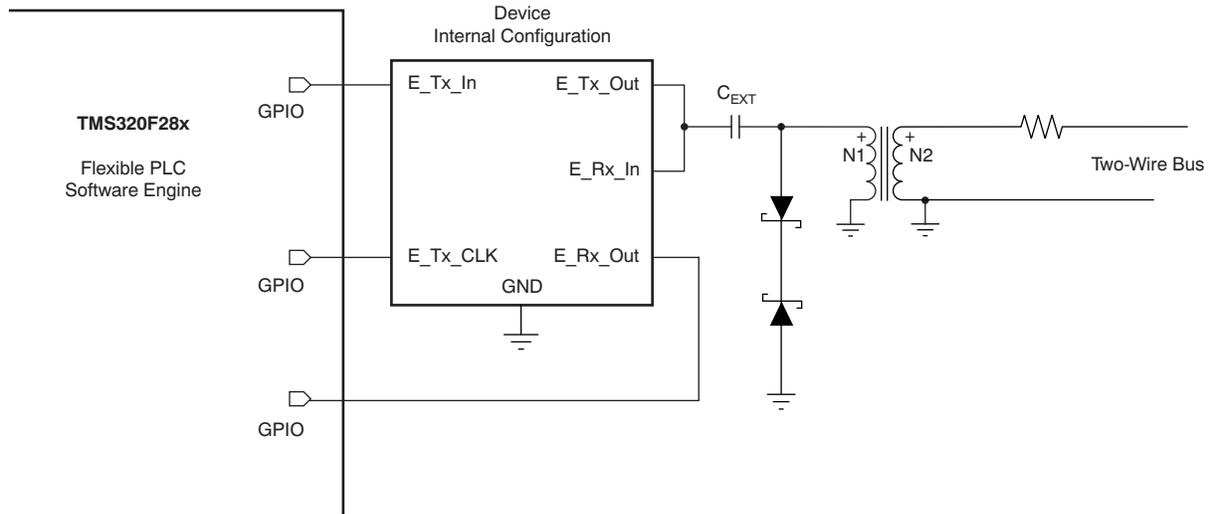
Figure 44. Typical Two-Wire Application for ETx and ERx
