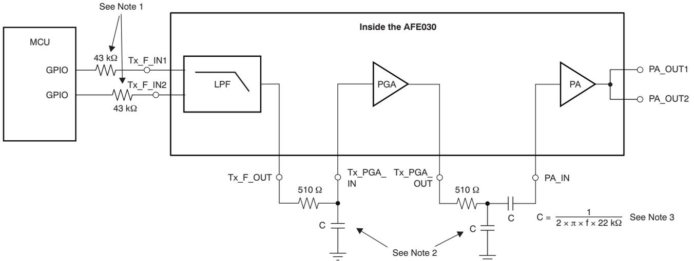
(1) When using both Tx Filter inputs, use 43-kΩ resistors to match the input resistance for best frequency response.
