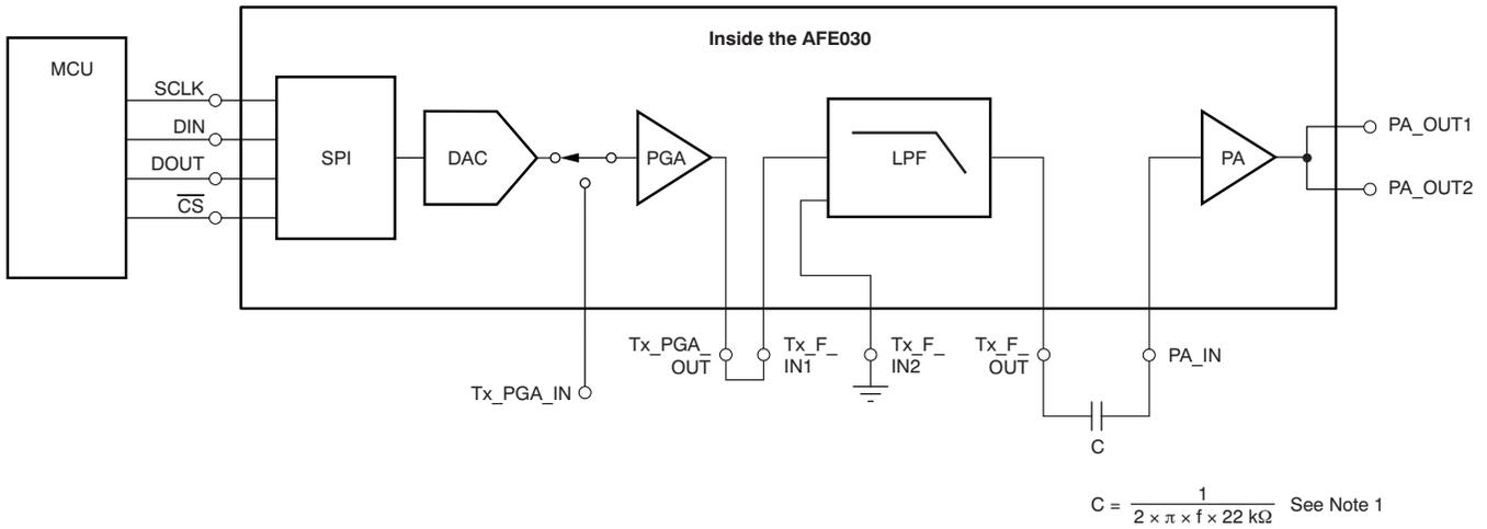
(1) For capacitor value C, f is the desired lower cutoff frequency and 22 kΩ is the PA input resistance.
