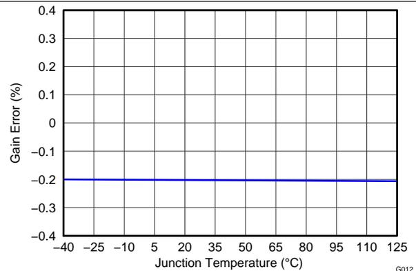
Figure 12. Rx PGA1 Gain Error vs Temperature
