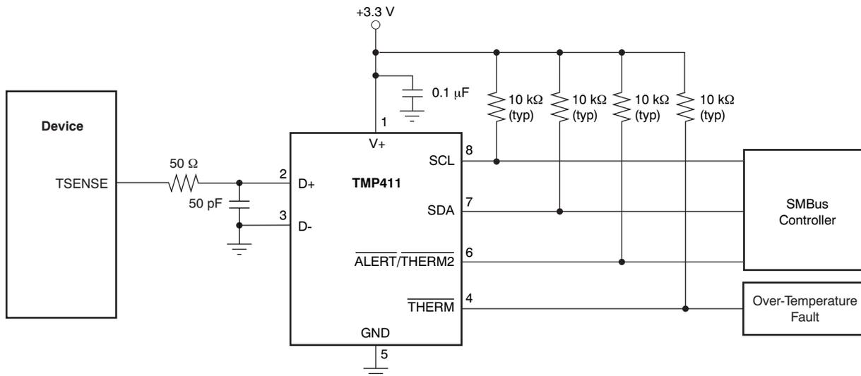
**Figure 45. Interfacing the TMP411 to the AFE030**
