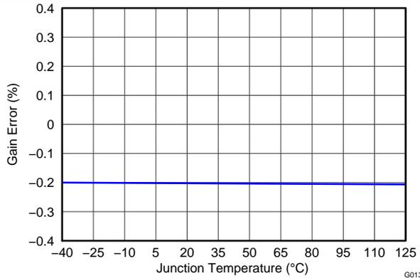
Figure 13. Rx PGA2 Gain Error vs Temperature
