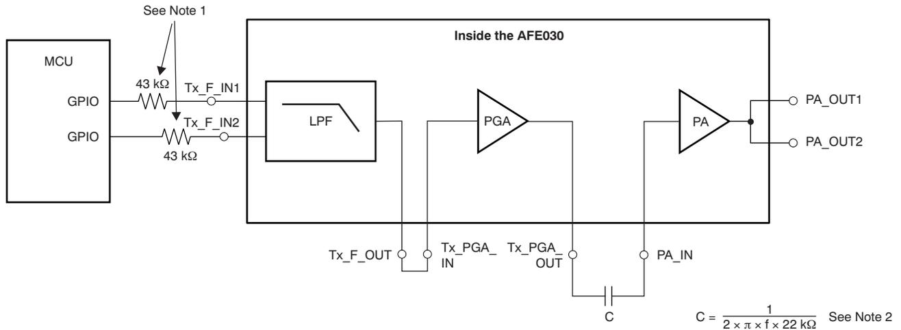
(1) When using both Tx Filter inputs, use 43-kΩ resistors to match the input resistance for best frequency response.
