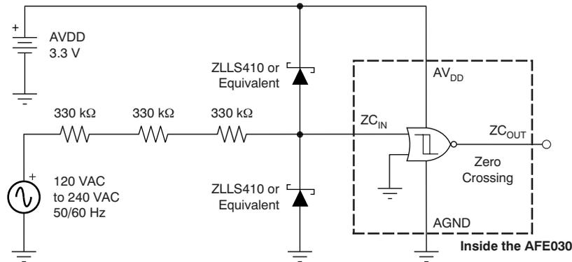
**Figure 38. Non-Isolated Zero Crossing Detection Using the AFE030**
