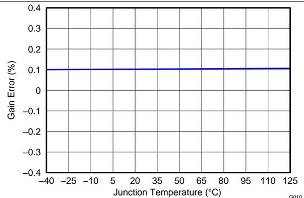
Figure 10. Tx PGA Gain Error vs Temperature
