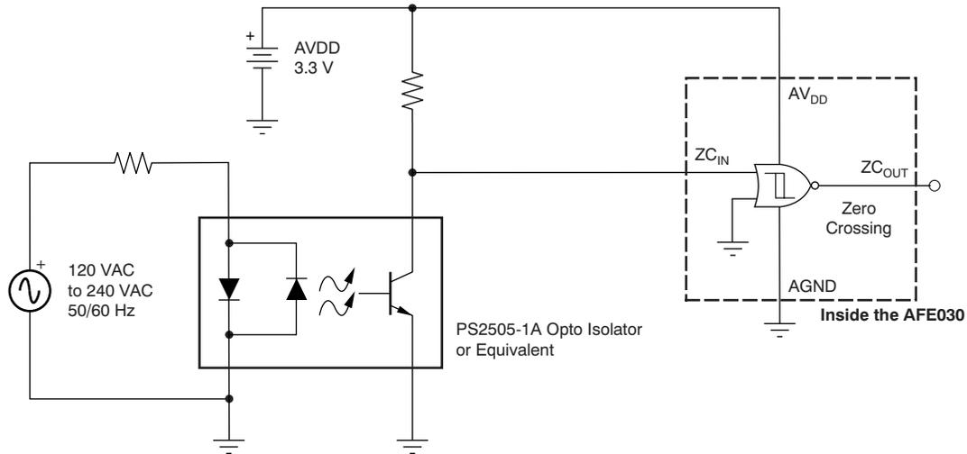
Figure 40. Isolated Zero Crossing Detection Using the AFE030
