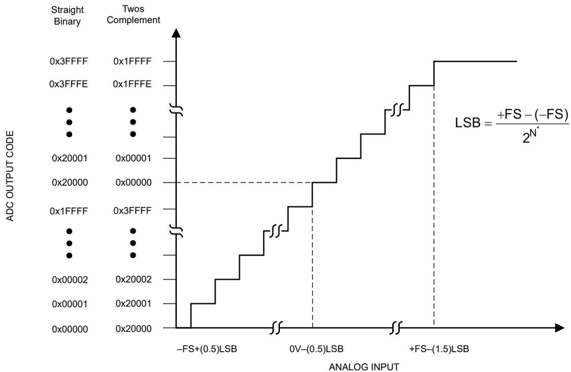
**Figure 6-3. Transfer Characteristics**
