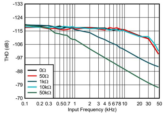
**Figure 5-25. THD vs Input Signal Frequency Across Source Impedance With Wide-Bandwidth LPF, RANGE =  $\pm 10V$**
