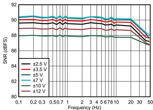
Figure 5-16. SNR vs Input Signal Frequency Across Input Ranges With Low-Bandwidth LPF
