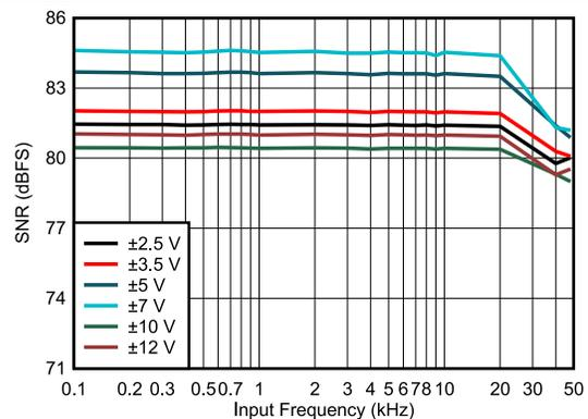
Figure 5-17. SNR vs Input Signal Frequency Across Input Ranges With Wide-Bandwidth LPF
