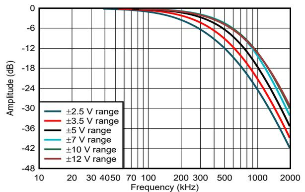
Figure 5-15. Wide-Bandwidth LPF Frequency Response Across Input Ranges
