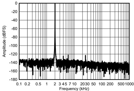
SNR = 90.2dBFS, THD = -117.6dB at  $f_{IN} = 2\text{kHz}$
