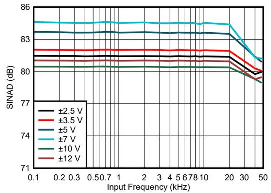
Figure 5-21. SINAD vs Input Signal Frequency Across Input Ranges With Wide-Bandwidth LPF
