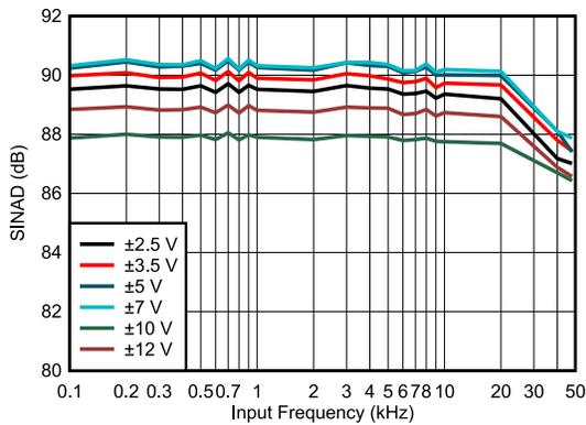
Figure 5-20. SINAD vs Input Signal Frequency Across Input Ranges With Low-Bandwidth LPF
