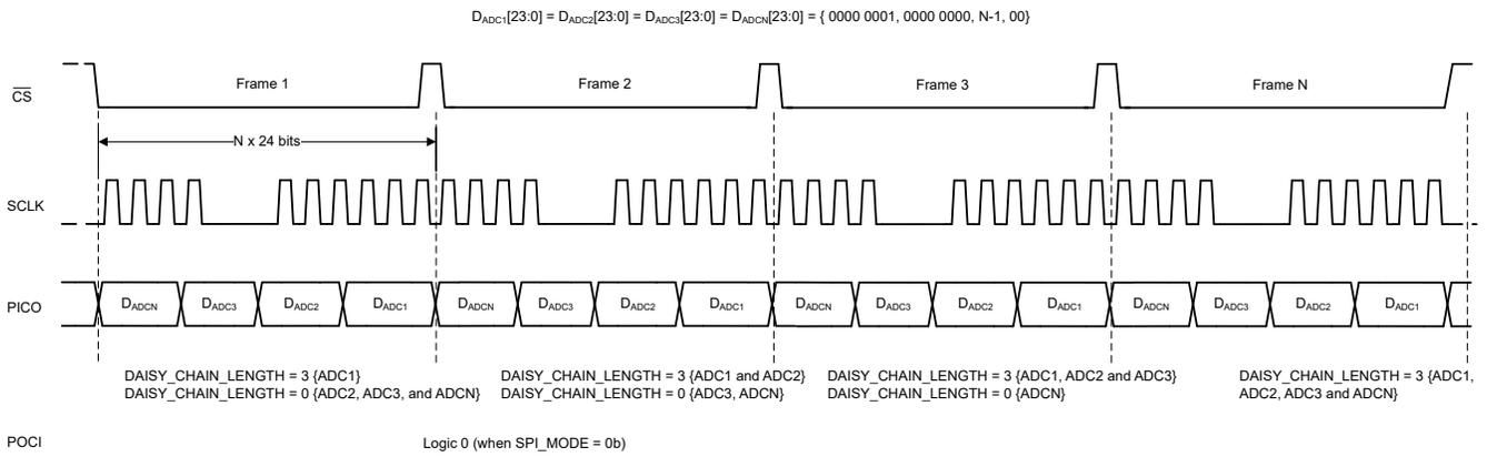
**Figure 6-13. Register Write to Configure the Daisy-Chain Length**
