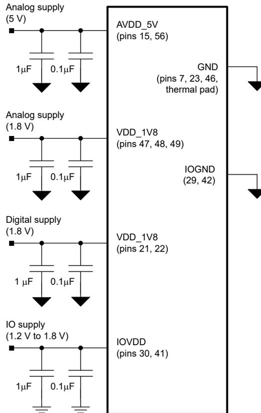
**Figure 8-4. Power-Supply Decoupling**
