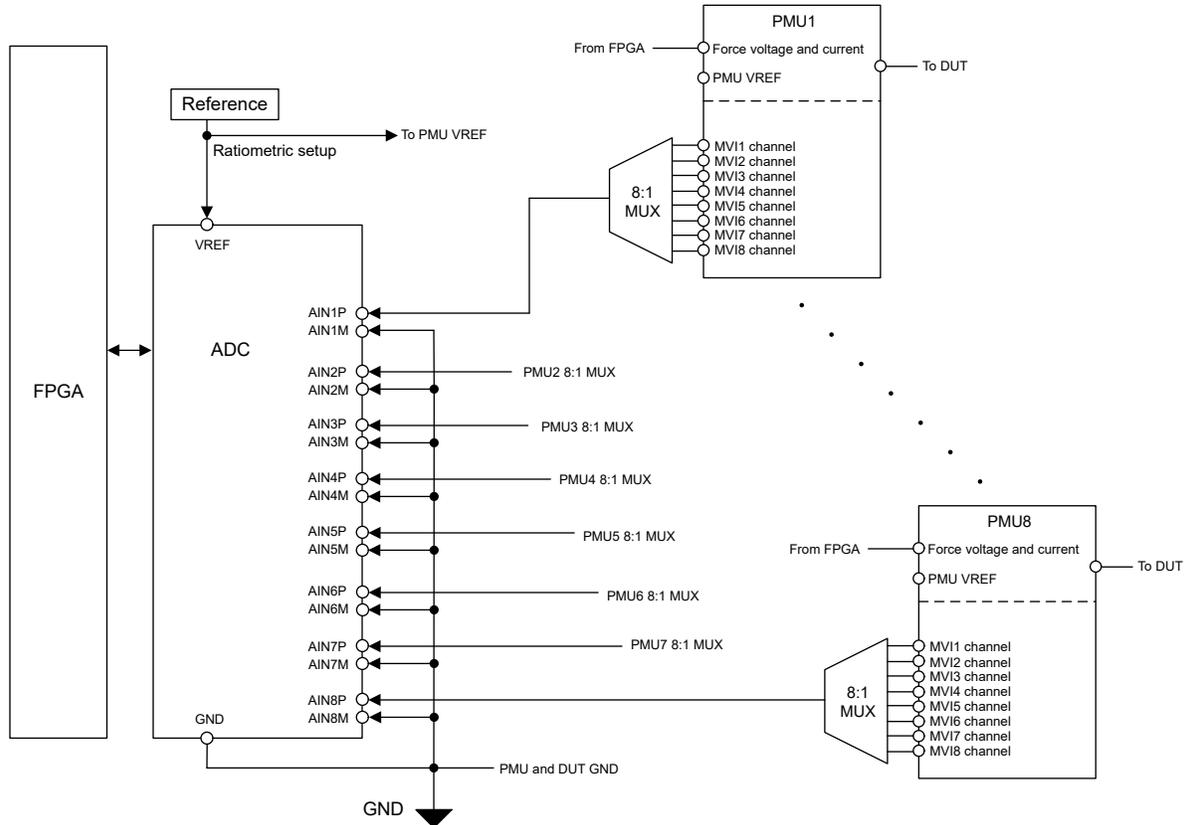
Figure 8-2. PMU With a Multiplexer
