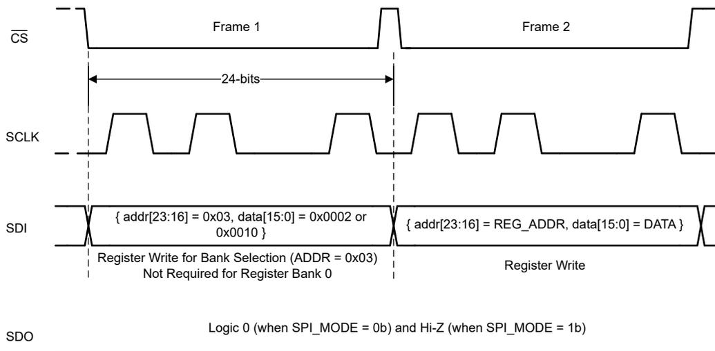
Figure 6-9. Register Write
