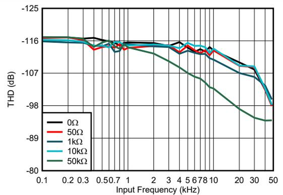
Figure 5-23. THD vs Input Signal Frequency Across Source Impedance With Wide-Bandwidth LPF, RANGE =  $\pm 5V$
