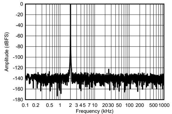
SNR = 83.7dBFS, THD = -121dB at  $f_{IN} = 2\text{kHz}$
