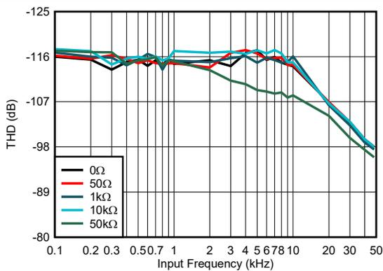
Figure 5-22. THD vs Input Signal Frequency Across Source Impedance With Low-Bandwidth LPF, RANGE =  $\pm 5V$
