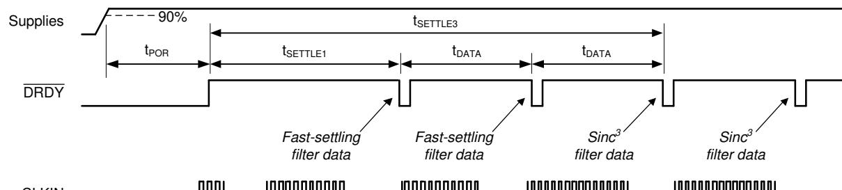
图 8-14. Fast Startup Behavior and Settling Times
