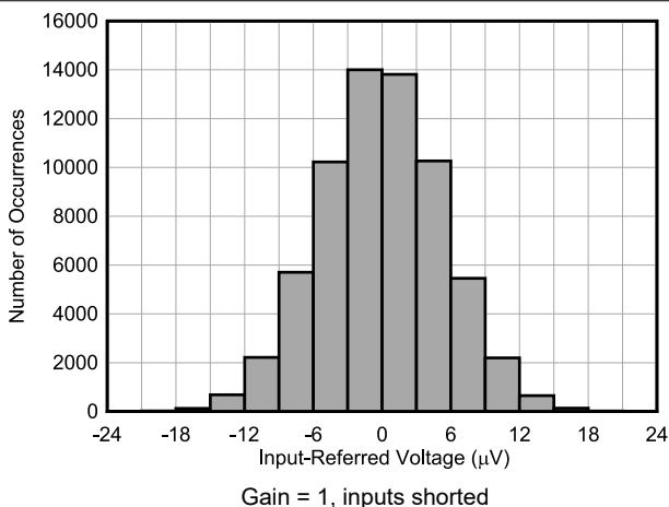
图 6-19. Single Device Noise Histogram at 32 kSPS
