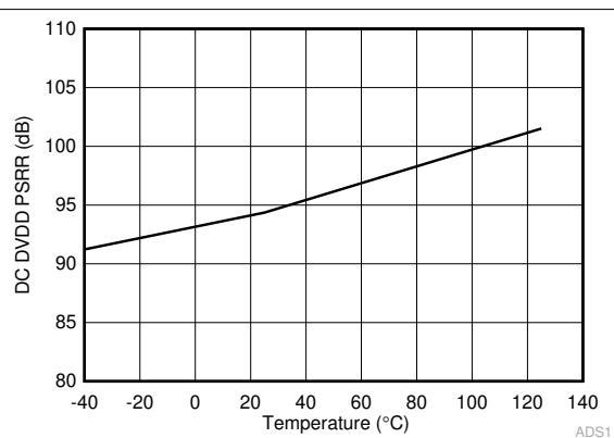
图 6-17. DC DVDD PSRR vs Temperature
