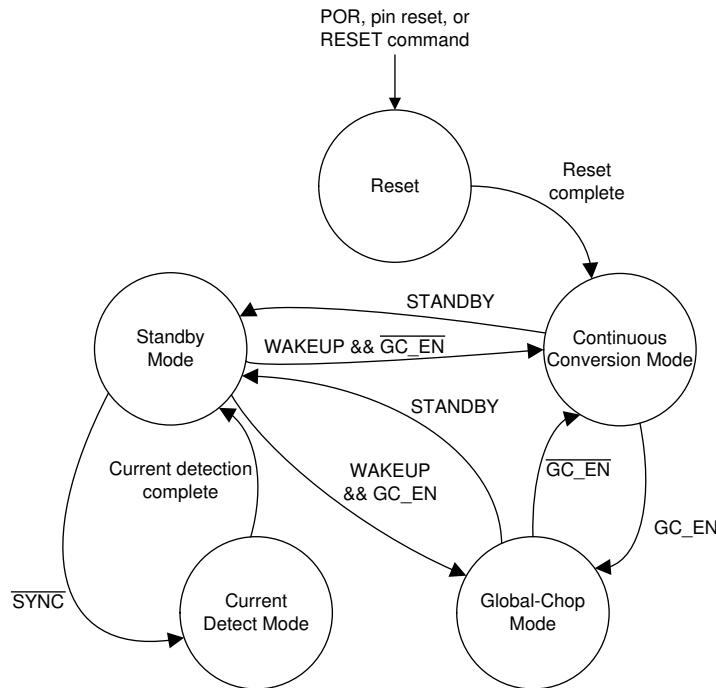
图 8-13. State Diagram Depicting Device Functional Modes
