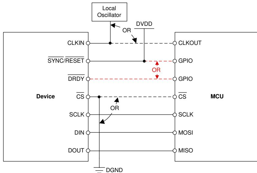
图 9-2. Minimum Connections Required to Operate the ADS131M02-Q1
