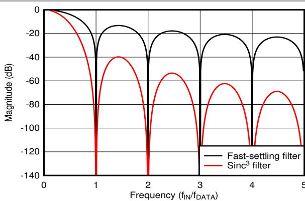
图 8-4. Fast-Settling and Sinc<sup>3</sup> Digital Filter Response
