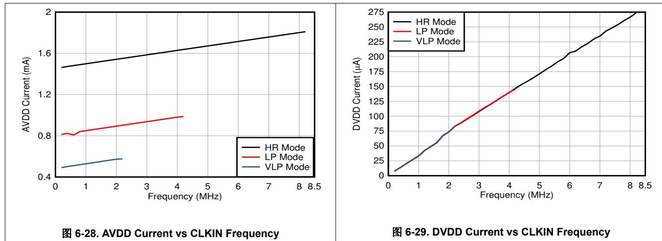
图 6-28. AVDD Current vs CLKIN Frequency
