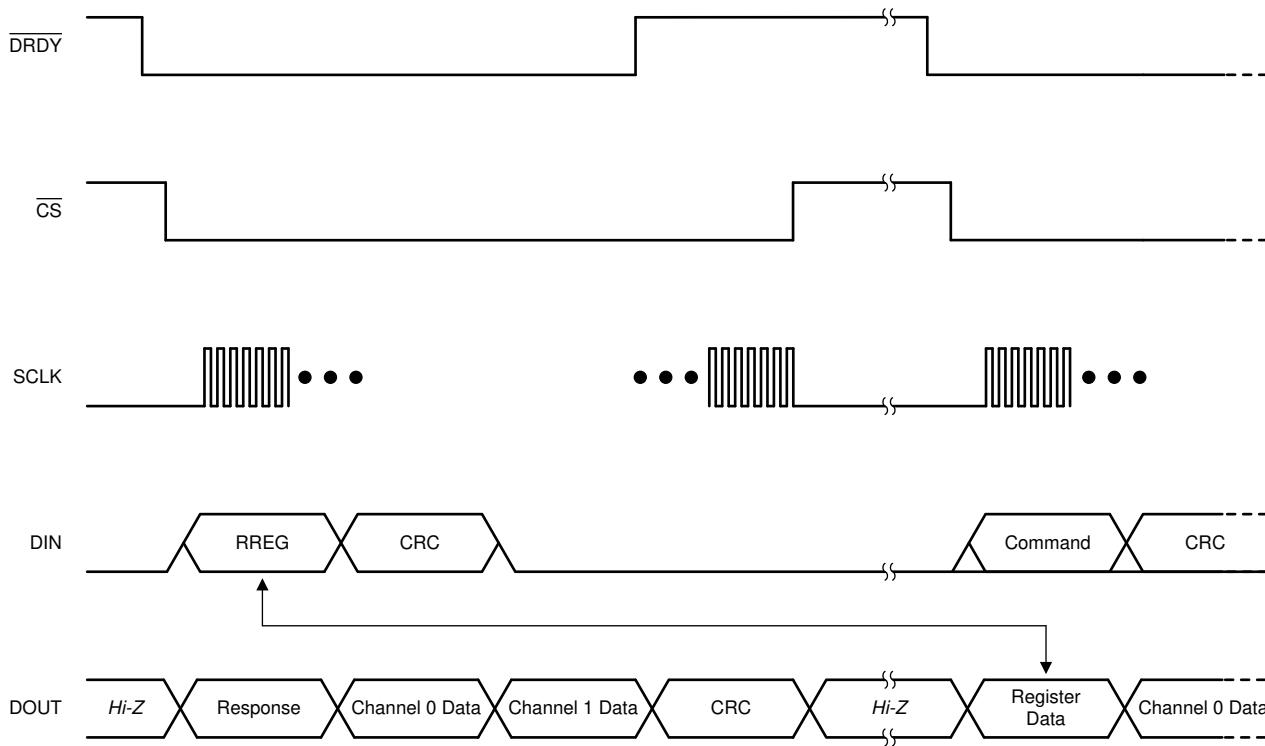
**图 8-23. Reading a Single Register**
