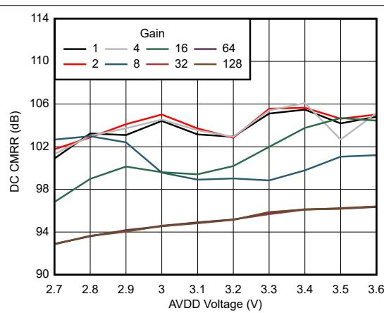
图 6-13. DC CMRR vs AVDD Voltage
