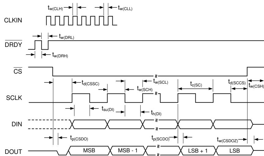
NOTE: SPI settings are CPOL = 0 and CPHA = 1. CS transitions must take place when SCLK is low.
