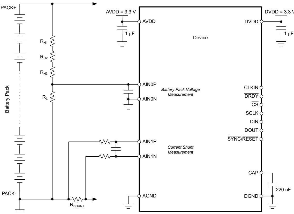
图 9-4. ADS131M02-Q1 in a Typical Battery Management System Application
