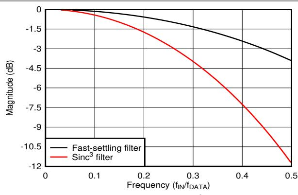
图 8-5. Fast-Settling and Sinc<sup>3</sup> Digital Filter Response, Pass-Band Detail
