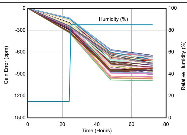
图 6-11. Gain Error vs Time Across Humidity
