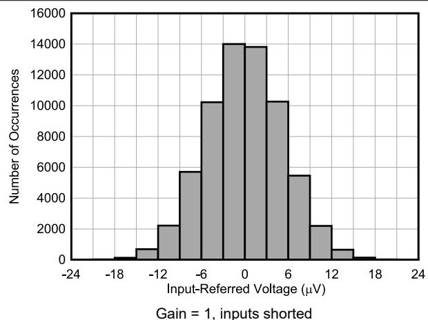
图 6-18. Single Device Noise Histogram at 4 kSPS
