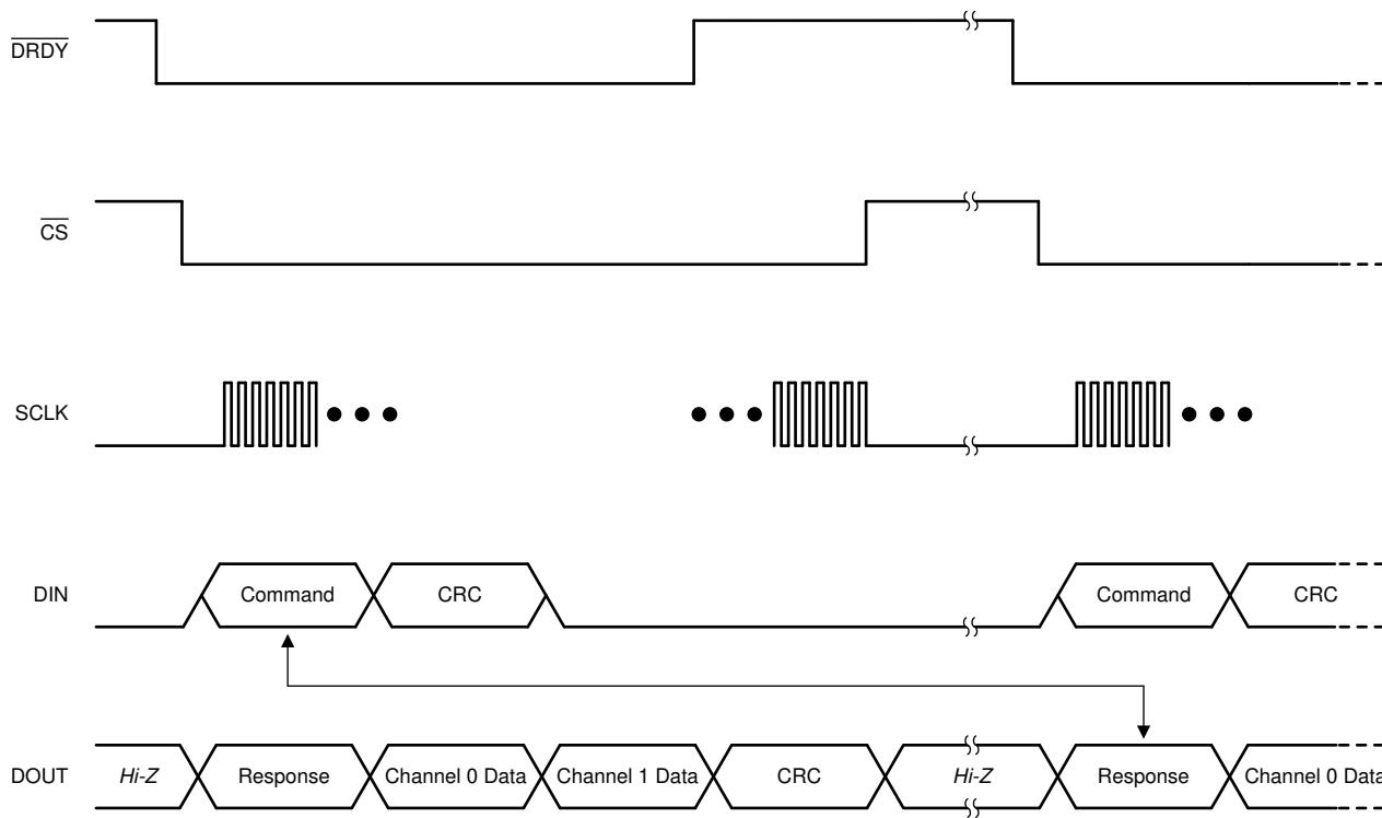
图 8-18. Typical Communication Frame
