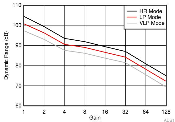
图 6-21. Dynamic Range at 4 kSPS vs Gain
