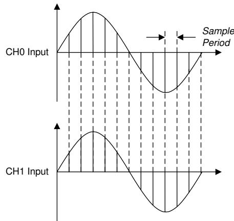
**图 8-9. Two Channel Outputs With Equal Phase Settings**
