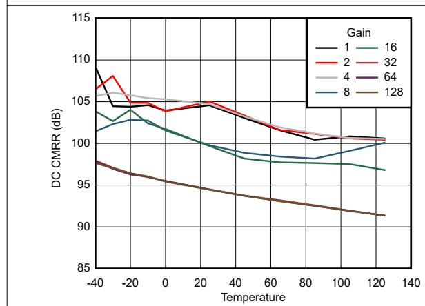
图 6-12. DC CMRR vs Temperature
