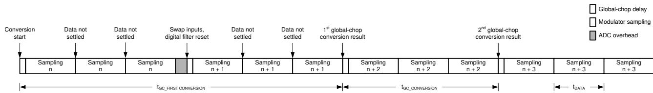
图 8-16. Conversion Timing With Global-Chop Mode Enabled
