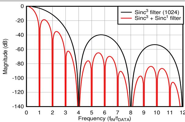
图 8-6. Digital Filter Response for OSR = 1024 and OSR = 4096
