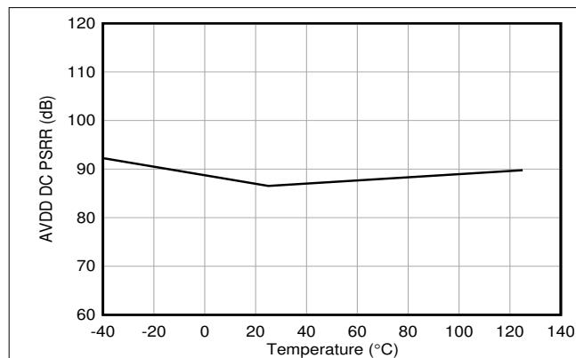
图 6-16. DC AVDD PSRR vs Temperature
