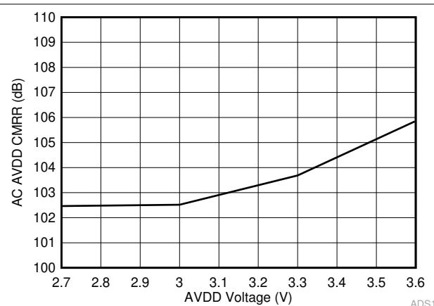
图 6-15. AC CMRR vs AVDD Voltage
