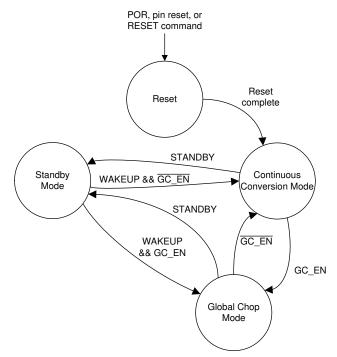
图 8-9. State Diagram Depicting Device Functional Modes
