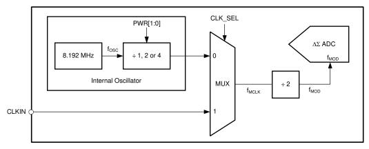
图 8-3. Main Clock Selection Diagram
