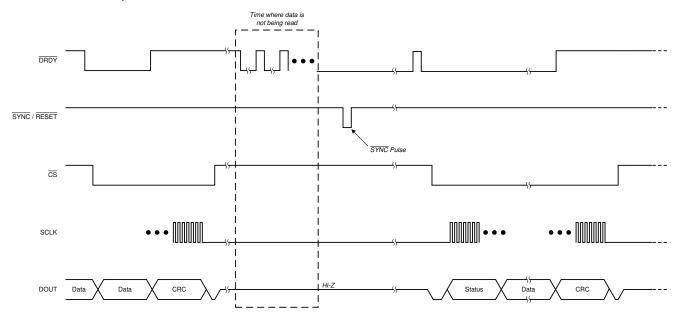
图 8-22. Collecting Data After a Pause in Data Collection Using the SYNC/RESET Pin
