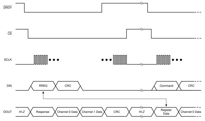
图 8-19. Reading a Single Register
