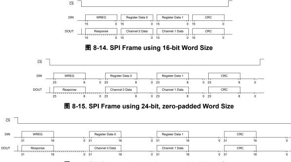
图 8-16. SPI Frame using 32-bit, zero-padded Word Size
