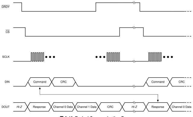
图 8-13. Typical Communication Frame
