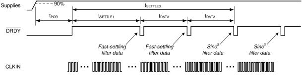
图 8-10. Fast Start-Up Behavior and Settling Times
