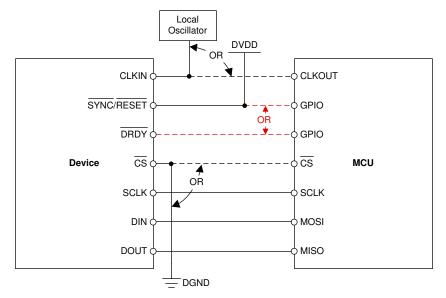
图 9-2. Minimum Connections Required to Operate the ADS130B02-Q1
