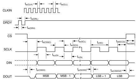
SPI settings are CPOL = 0 and CPHA = 1.  $\overline{CS}$  transitions must take place when SCLK is low.
